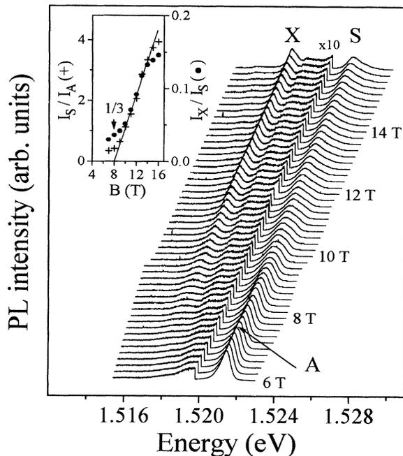
FIG. 1. cw photoluminescence spectra of sample I, with density (under photoexcitation)  $p \approx 6.2 \times 10^{10} \text{ cm}^{-2}$ , at  $T_{\text{bath}} = 60 \text{ mK}$  and for magnetic fields  $B = 0 - 16 \text{ T}$  in  $0.2 \text{ T}$  steps. The low energy parts of the spectra are multiplied by a factor of 10 to show the appearance of line X. Inset shows the ratios of the line intensities.
