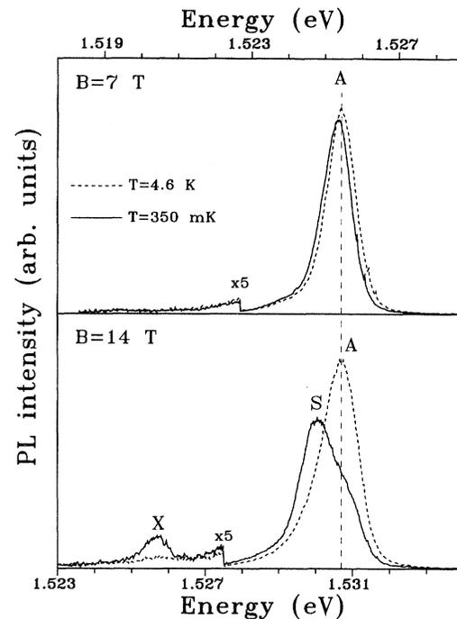
FIG. 2. cw photoluminescence spectra of sample II, with density (under photoexcitation)  $p \approx 7.1 \times 10^{10} \text{ cm}^{-2}$ , at  $T = 350 \text{ mK}$  and  $4.6 \text{ K}$ . Upper (lower) part of the figure shows the spectra at  $B = 7 \text{ T}$  ( $14 \text{ T}$ ).
