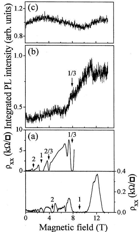
FIG. 4. Magnetic field dependence of (a) the resistivity  $\rho_{xx}$  after cooling in the dark (lower trace) and under photoexcitation (upper trace); (b) PL intensity integrated over energy and over the time interval  $t=5$ –30 ns; (c) PL intensity integrated over energy and over all time. The data in (b) are normalized to the total intensity shown in (c), and thus represent the relative fraction of the long-time recombination.
