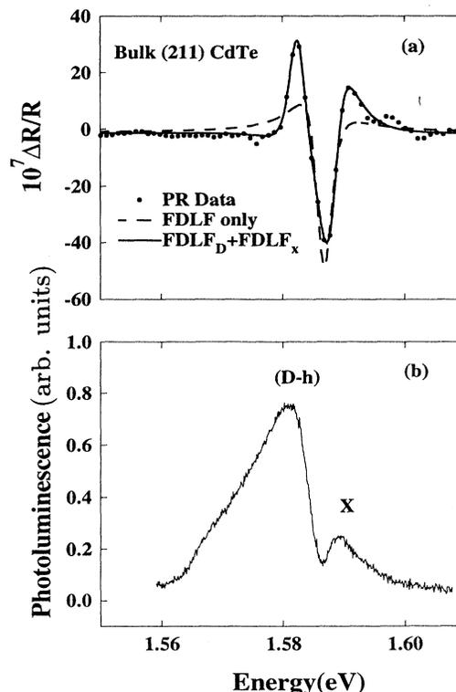
FIG. 1. PR and PL spectra from undoped bulk (211) CdTe at 80 K. (a) PR line-shape analysis using a single transition (dashed line) gives a poor fit, while that using two transitions (solid line) yields energies of 1.582 (donor) and 1.587 eV (free exciton). (b) The PL spectrum clearly shows the donor-hole ( $D, h$ ) and free exciton ( $X$ ) recombination.
