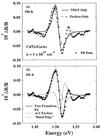
FIG. 3. PR from the CdTe:I/GaAs epilayer at 296 K. (a) PR line-shape analysis with a single band-to-band (solid line) or exciton (dashed line) transition results in a poor fit to the data. (b) A two-transition fit which includes an exciton transition and a general Lorentzian function representing near-edge transitions. The relative contributions are indicated.
