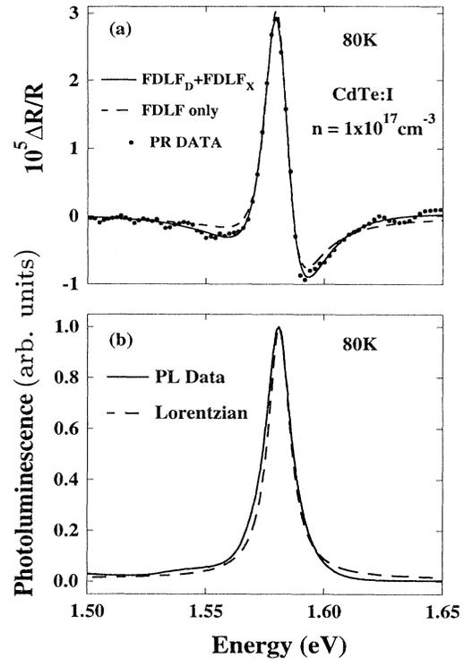
FIG. 2. PR and PL spectra from CdTe:I epilayer ( $n \sim 1 \times 10^{17} \text{ cm}^{-3}$ ) at 80 K. (a) PR line-shape analysis with only the ( $D, h$ ) transition (dashed line), and the improved fit obtained with a contribution from free excitons (solid line). (b) PL dominated by ( $D, h$ ) emission at 1.581 eV, and the predicted PL spectrum (dashed line) generated using parameters from PR analysis.
