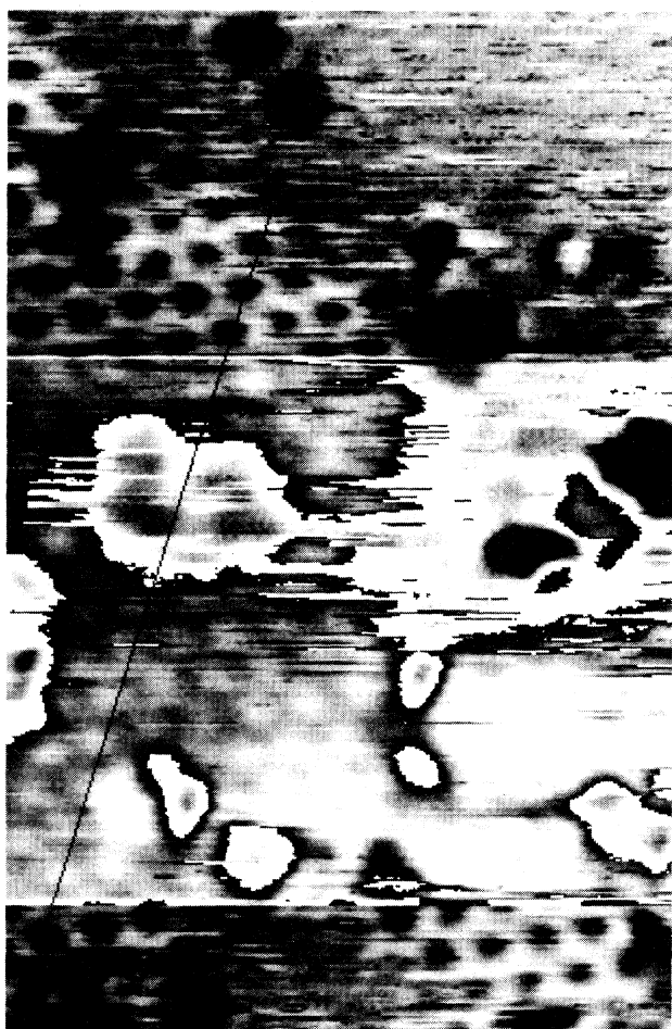
FIG. 4. Scanning-tunneling-microscopy image of a medium coverage Na covered surface, where a \sqrt{3} island is imaged under different tunneling conditions. The upper and lower part shows the inverted imaging of the \sqrt{3} structure, induced by approaching the tip further to the surface. Na atoms appear as depletions in these STM images ( \Theta=0.14 , I_t=32 \text{ nA} , V_t=-0.4 \text{ V} in the upper and lower part, V_t=-0.6 \text{ V} in the middle, 62 \times 100 \text{ \AA}^2 ).
