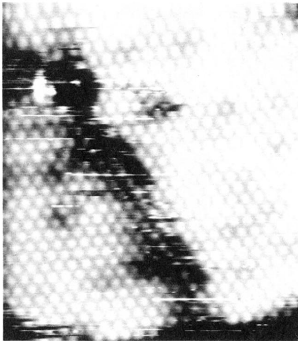
FIG. 7. Scanning-tunneling-microscopy topograph of two \sqrt{3} islands which are separated by a "light wall." The streaks are due to fast exchange of atoms between the two islands ( \Theta=0.30 , I_t=3.0 nA, V_t=-1.2 V, 110 \times 124 \text{ \AA}^2 ).
