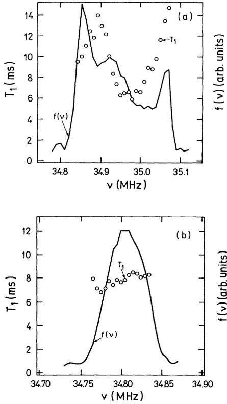
FIG. 1. (a) Variation of <sup>35</sup>Cl NQR  $T_1$  over the inhomogeneous <sup>35</sup>Cl NQR line  $f(\nu)$  in incommensurate BCPS at 90 K. The experimental NQR line shape can be described by expressions (2a)–(2d) with  $\nu_2 \approx 2\nu_1$ . (b) Variation of the <sup>35</sup>Cl NQR  $T_1$  over the NQR line shape in incommensurate BCPS at 140 K.
