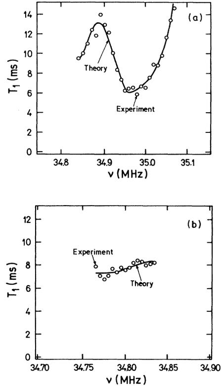
FIG. 3. (a) Comparison between the theoretical and the experimentally observed variation of the  $^{35}\text{Cl}$   $T_1$  over the NQR line in BCPS at 90 K. (b) Comparison between the theoretical and experimentally observed variation of the  $^{35}\text{Cl}$   $T_1$  over the NQR line in BCPS at 140 K.
