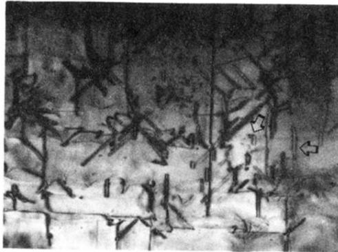
FIG. 8. Contrast inside and outside the dislocation loops in the superlattice ( g=2\bar{2}0 and \bar{2}20 ).
