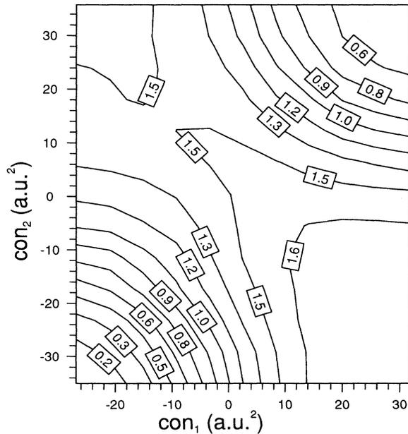
FIG. 6. Contour plot of the energy barrier,  $E_1$  eV, to kink pair activation for the  $90^\circ$   $\beta$  partial in GaAs.
