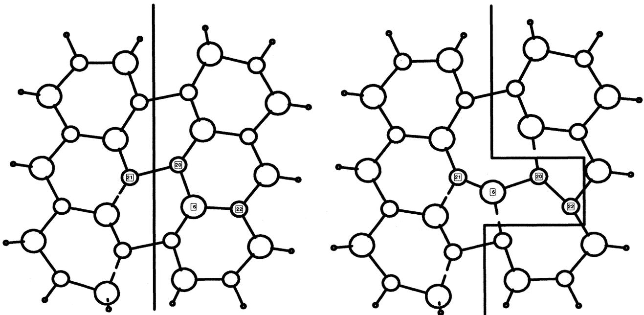
FIG. 3. The atoms in the glide (111) plane, i.e., parallel to the horizontal plane in Fig. 1, for the relaxed straight and kinked 158 atom GaAs cluster. The full line in the first figure is in the dislocation core along  $[10\bar{1}]$  and is perpendicular to the partial Burgers vector of the  $90^\circ$  partial along  $[1\bar{2}1]$ . The double kink has moved part of the dislocation in the (111) slip plane and in the direction of the Burgers vector.
