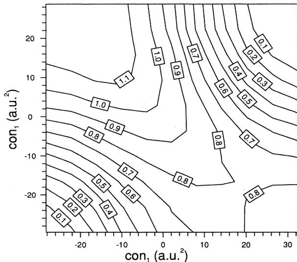
FIG. 8. Contour plot of the energy barrier,  $E_1$  eV, to kink pair activation for the  $90^\circ$   $\alpha$  partial in GaAs. The lowest left hand corner is close to a configuration of a straight dislocation and the upper right hand corner is close to that of the double kink.
