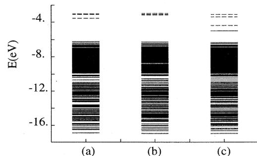
FIG. 5. Cluster energy levels (eV) for the (a) straight (b) kinked, and (c) saddle point dislocation structures in Si. The broken lines show the three lowest unoccupied levels. Note that there is a substantial energy gap between the filled and empty levels for the straight and kinked dislocation but two deep gap levels for the saddle point configuration corresponding to double kink activation.
