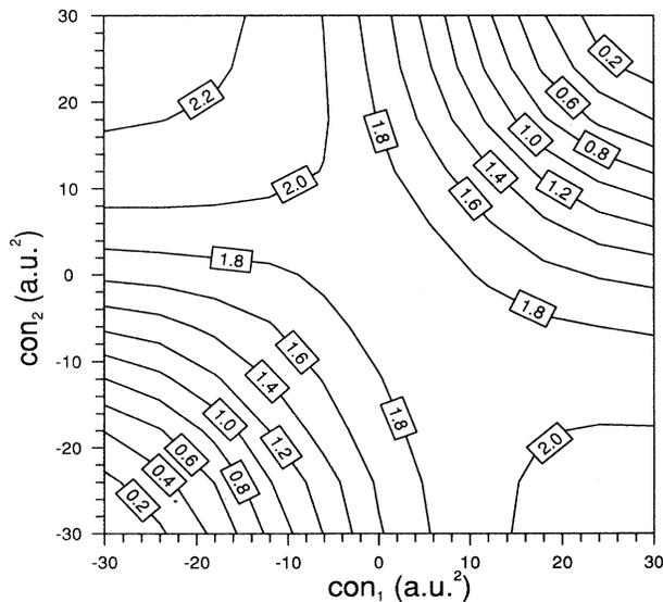
FIG. 4. Contour plot of the energy barrier,  $E_1$  eV, to kink pair activation for the  $90^\circ$  partial in Si. The lower left hand corner is close to the configuration of the straight dislocation, whereas the upper right hand corner is close to that of the double kink.
