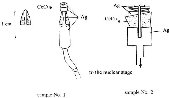
FIG. 1. Sketch of the  $\text{CeCu}_6$  samples used in this work and their thermal connection to the nuclear stage.
