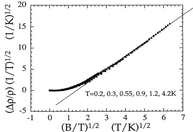
FIG. 5.  $(\Delta\rho/\rho)(T)^{-1/2}$  as a function of  $(B/T)^{1/2}$  showing a universal curve characteristic of electron-electron interaction effects.
