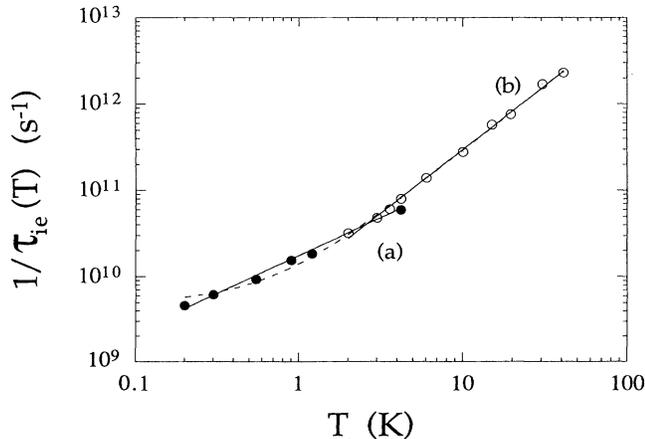
FIG. 4. Temperature dependence of  $1/\tau_{ie}$  between 200 mK and 30 K (solid circles, our data; open circles, data from Ref. 11). The solid lines are (a)  $1.9 \times 10^{10} T^{0.87}$  and (b)  $1.0 \times 10^{10} T^{1.47}$ , the dashed line is a fit to a  $A_0 + A_1 T^{1.5}$  law.
