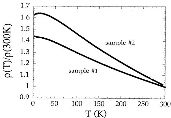
FIG. 1. Temperature dependence of the resistivity of AlCuFe quasicrystalline thin films, sample no. 1,  $\rho_{300 \text{ K}} \sim 2000 \mu\Omega$  cm; and sample no. 2,  $\rho_{300 \text{ K}} \sim 2700 \mu\Omega$  cm.
