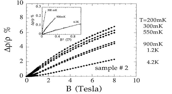
FIG. 2. Magnetoresistance (MR) of an AlCuFe quasicrystalline thin film; lines are guides for the eye. In the inset MR as a function of  $B^2$  in the low-field limit. The solid lines are linear fits using equation  $\Delta\rho/\rho = \rho\alpha(T)B^2$ .
