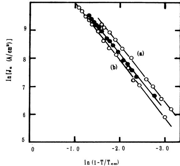
FIG. 5. Logarithmic plots of  $J_c(T)$  in a temperature range close to  $T_{cm}$ . curve a: 0.5 T; solid circles: 1.0 T; curve b: 2.0 T.
