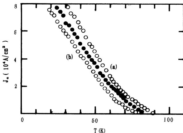
FIG. 4. Temperature dependence of critical current density  $J_c(T)$  at several magnetic fields; curve a: 0.5 T; solid circles: 1.0 T; curve b: 2.0 T.
