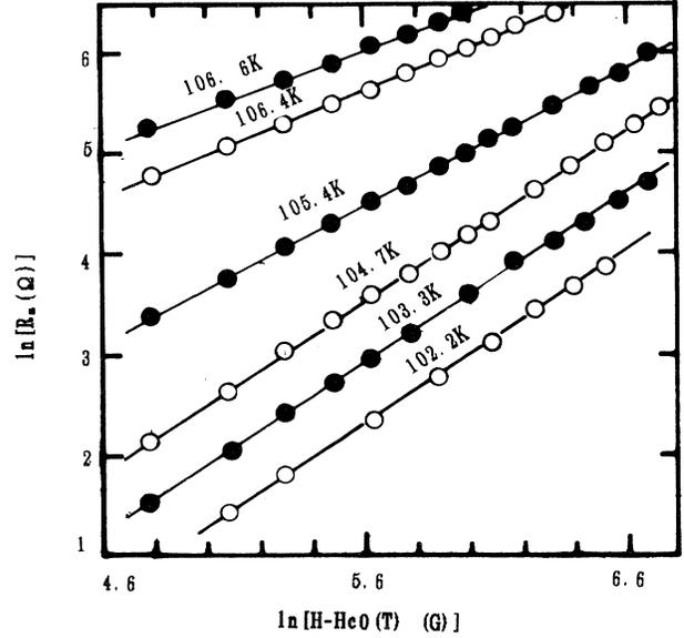
FIG. 2. Magnetoresistance curves of the Bi-2223 film itself for  $H \perp I$  in logarithmic plots of  $R_s$  versus  $(H - H_{c0})$ , where  $H_{c0}$  is the field above which the magnetoresistivity appears.
