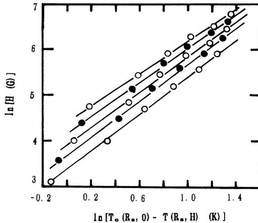
FIG. 3. Temperature width versus magnetic field for several fixed resistivity levels in logarithmic plots. From the top to the bottom, the lines are related to the resistance levels 50, 40, 30, 20, and  $10 \mu\Omega$ .
