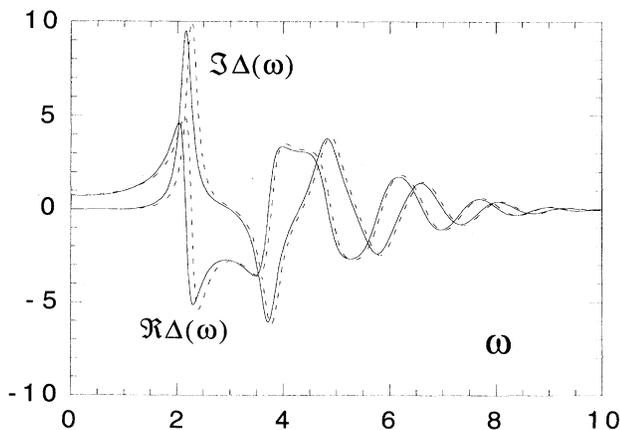
FIG. 5.  $\text{Re}[\Delta(\omega)]$  and  $\text{Im}[\Delta(\omega)]$  from numerical integration of Eq. (31) (solid line) and from the approximate equation Eq. (38) (dashed line), for  $T/T_c=0.3$ .
