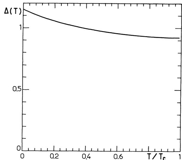
FIG. 7. Frequency location  $\Delta(T)$  of the maximum of the density of states  $N(\omega)$  as a function of reduced temperature.
