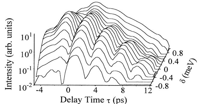
FIG. 4. Spectrally resolved DFWM signal. The detuning  $\delta$  corresponds to the difference between the detection energy and the biexciton resonance.
