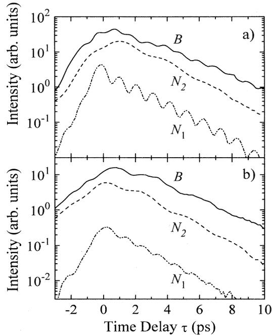
FIG. 2. Time-integrated DFWM intensity versus delay  $\tau$  for (a) parallel and (b) cross-polarized laser fields. Solid line: excitation  $B$  (broadband, between lh and hh); dashed line: excitation  $N_2$  (narrow band, between hh and BX); dotted line: excitation  $N_1$  (narrow band, between lh and hh).
