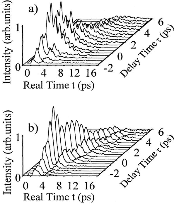
FIG. 5. Measured intensity of the TR-DFWM signal at various probe delays for (a) parallel and (b) cross-polarized laser fields.
