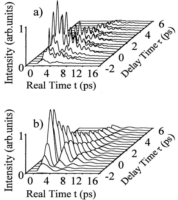
FIG. 7. Calculated intensity of the TR-DFWM signal at various probe delays based on the ten-level model for (a) parallel and (b) cross-polarized fields under excitation condition  $B$  and the same parameters as in Fig. 6, except the local field parameter:  $L = 0.1$  meV.
