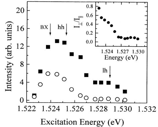
FIG. 3. Peaks of the TI-DFWM signals for PP (closed squares) and CP (open circles) polarizations versus excitation energy. Inset: The ratio of the PP and CP TI-DFWM intensity for different excitation energies (probe delay  $\tau = 0$ ).
