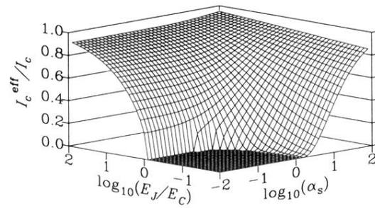
FIG. 1.  $I_c^{\text{eff}}$  calculated in the adiabatic limit  $\Delta/E_C \rightarrow \infty$  for  $\varphi_0 = 0$ , normalized by the classical value  $I_c = 2eE_J$ .
