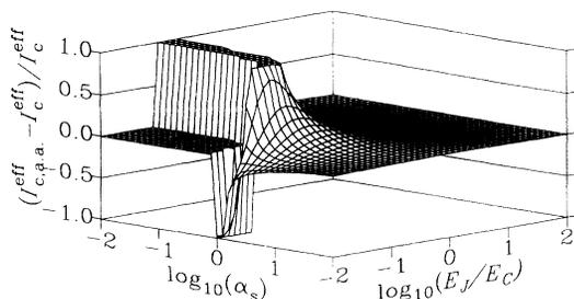
FIG. 3. Relative deviation of the critical current in the adiabatic approximation,  $I_{c,\text{a.a.}}^{\text{eff}}$ , from the nonadiabatic result  $I_c^{\text{eff}}$  as a function of  $E_J/E_C$  and  $\alpha_s$  for  $\Delta/E_C = 0.1$  and  $\varphi_0 = 0$ . The graph is clipped at  $\pm 1$ .
