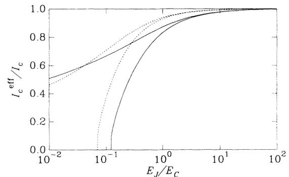
FIG. 5. Dependence of  $I_c^{\text{eff}}$  on the ratio of Josephson energy and charging energy, for  $\Delta/E_C = 0.1$  and  $\varphi_0 = 0$ . The solid curve is the nonadiabatic SCHA result, and the dashed curve the adiabatic approximation;  $\alpha_s = 10$  for the upper pair of curves, and  $\alpha_s = 0.5$  for the lower pair.
