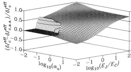
FIG. 4. Relative deviation of the suppression of the critical current in the adiabatic limit,  $\delta I_{c,\text{a.a.}} \equiv I_{c,\text{a.a.}}^{\text{eff}} - I_c$ , from the nonadiabatic SCHA result  $\delta I_c \equiv I_c^{\text{eff}} - I_c$ , for  $\Delta/E_C = 0.1$  and  $\varphi_0 = 0$ .
