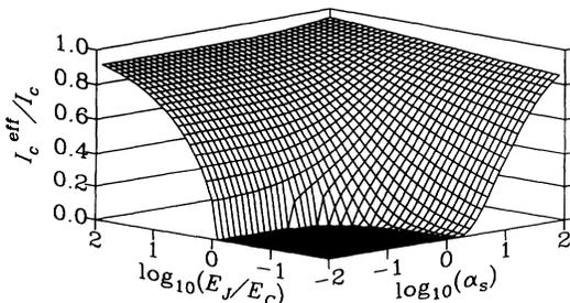
FIG. 1.  $I_c^{\text{eff}}$  calculated in the adiabatic limit  $\Delta/E_C \rightarrow \infty$  for  $\varphi_0 = 0$ , normalized by the classical value  $I_c = 2eE_J$ .
