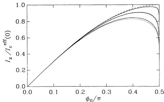
FIG. 7. Supercurrent-phase relation, normalized by  $I_c^{\text{eff}}(\varphi_0 = 0)$ . The solid curves are the nonadiabatic SCHA results, the dashed curves the adiabatic approximation. The three pairs of curves correspond to (from top to bottom)  $E_J/E_C = 10$ ,  $E_J/E_C = 1$ , and  $E_J/E_C = 0.1$ ;  $\alpha_s = 10$  and  $\Delta/E_C = 0.1$  for all pairs. The topmost curve (with long dashes) is the classical Josephson relation  $I_x/I_c = \sin \varphi_0$ .
