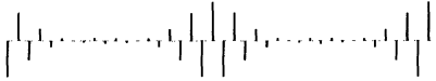
FIG. 5. Finite time evolution seen in a MD simulation of the predicted fastest growing ZBM instability perturbation in a 40-particle (k_2, k_4) lattice, with periodic boundary conditions. The anharmonicity parameter is \Lambda_4=0.0067 , and the unperturbed ZBM amplitude is A=0.015a . The ZBM was seeded with the velocity and position perturbations predicted by our RWA stability analysis for the fastest growing ZBM instability perturbation, which occurs for (k_p a)_{\max}=0.10\pi . The maximum amplitude for the perturbation seed is 1% of the unperturbed ZBM amplitude. The figure gives longitudinal displacements at the oscillation maximum; they are plotted in the vertical direction for clarity. The same vertical unit is used in each panel.
