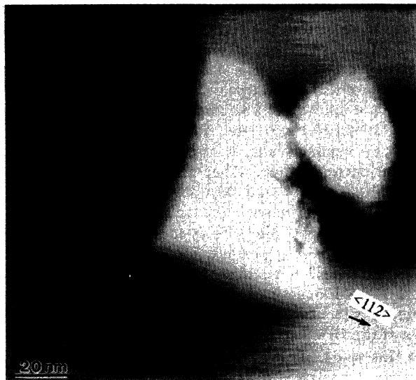
FIG. 1. HTSTM image at 710^\circ\text{C} in constant-current mode. Scanning area is 100\times 100\text{ nm}^2 , sample bias voltage -0.84\text{ V} , and tunneling current 0.2\text{ nA} .
