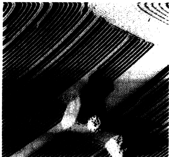
FIG. 2. HTSTM image at 690^\circ\text{C} in constant-height mode. Scanning area is 200\times 200\text{ nm}^2 , sample bias voltage -1.22\text{ V} , and tunneling current 0.09\text{ nA} .
