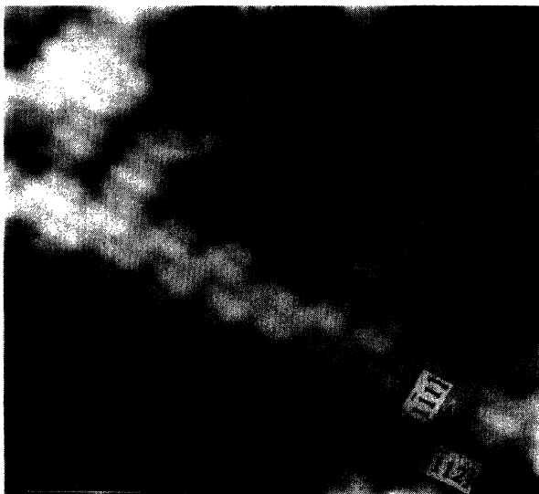
FIG. 6. STM image of a filled state of the connection between the 16 \times 2 and the (17,15,1) 2 \times 1 structures at room temperature in constant-current mode. Scanning area is 10 \times 10 \text{ nm}^2 , sample bias voltage -0.78 \text{ V} , and tunneling current 0.3 \text{ nA} .
