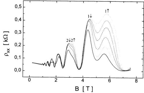
FIG. 2. Longitudinal resistivity  $\rho_{xx} = \epsilon_x / j_x$  vs magnetic field up to 8 T for several fixed channel currents (sample CS50/7,  $T = 1.3$  K).  $I = 1 \mu\text{A}$  (solid);  $I = 1.5 \mu\text{A}$  (dot);  $I = 2 \mu\text{A}$  (dash);  $I = 2.5 \mu\text{A}$  (dash dot);  $I = 3 \mu\text{A}$  (short dash);  $I = 4 \mu\text{A}$  (short dot).
