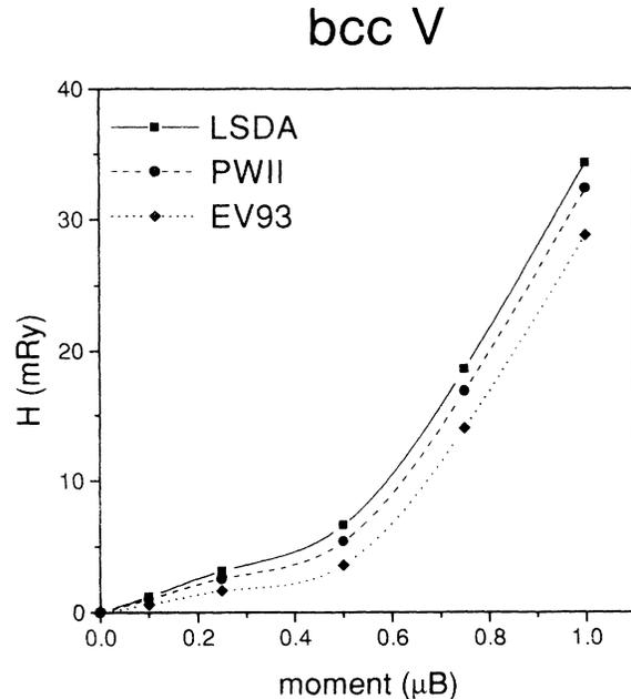
FIG. 3. Stabilizing field  $H$  (in mRy) as function of moment based on a FSM calculation for V using the three models.
