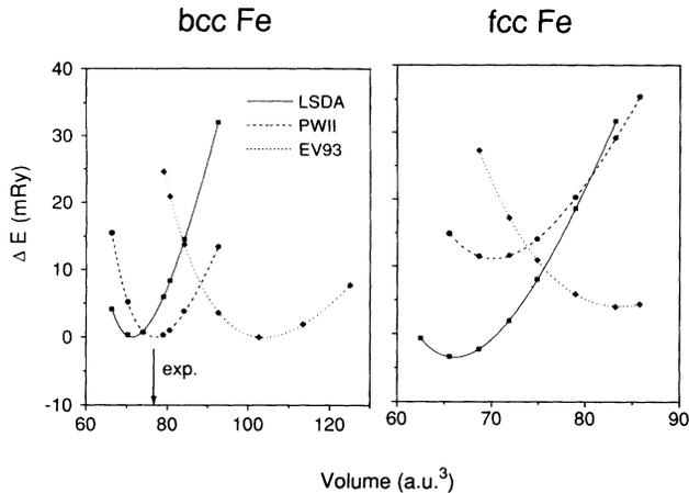
FIG. 1. Total energy (mRy) of Fe (with respect to the bcc equilibrium) in the bcc (left panel) and fcc (right panel) structure as a function of volume for LSDA (squares, solid line), PWII (circles, dashed line), and EV93 (diamonds, dotted line).
