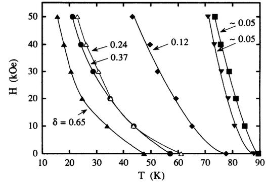
FIG. 3. Vortex-glass phase boundaries determined for YBCO films with  $\delta=0.65, 0.37, 0.12, 0.05$ , and  $0.05$ .
