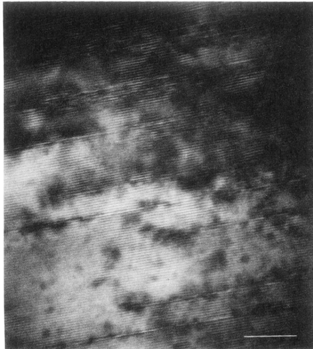
FIG. 6. Lattice fringe image corresponding to the [100] zone axis of a region close to that shown in Fig. 5. Note the high density of stacking faults. Scale bar corresponds to 25 nm.
