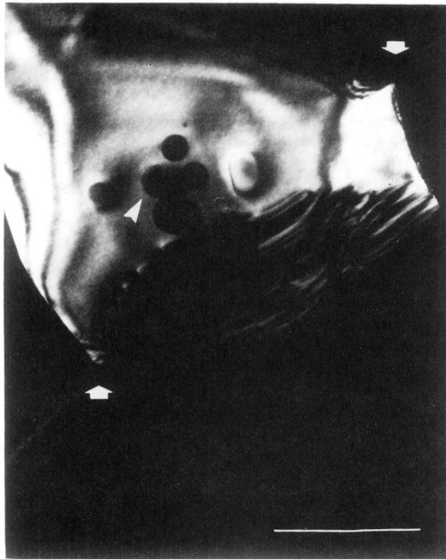
FIG. 9. TEM image of a 2:1:1 precipitate intercepted by a microcrack at places arrowed in the figure. The region between both intercepts shows a complex dislocation network. The arrowhead indicates Y 2 O 3 inclusions. The scale bar corresponds to 0.5 \mu\text{m} .
