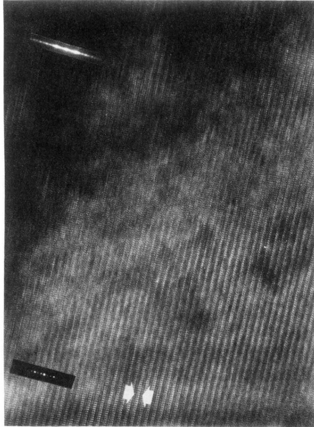
FIG. 4. HRTEM image viewed along the [100] direction showing a transition from a well-ordered zone (left-hand side) to a highly defective one (right-hand side of the micrograph) in the 1:2:3 matrix along its associated SAD patterns. Distance between arrow tips equals 1.17 nm.
