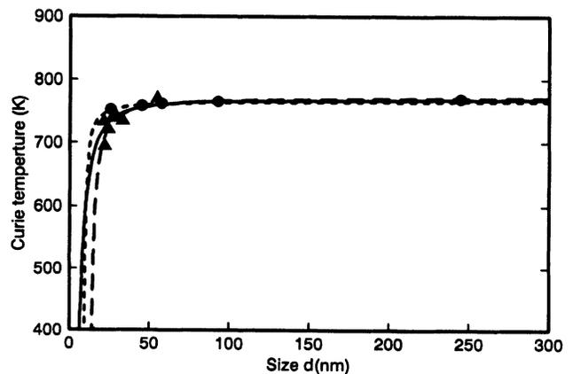
FIG. 9. Size dependence of the  $T_C$  of PbTiO<sub>3</sub> particles.
