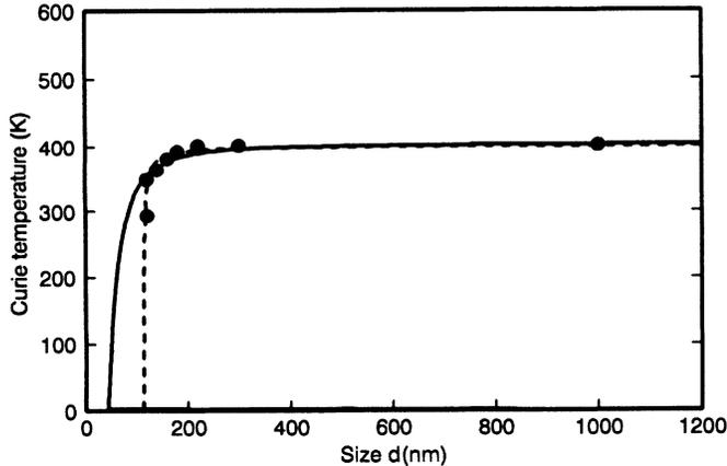
FIG. 10. Size dependence of the  $T_C$  of  $\text{BaTiO}_3$  particles.
