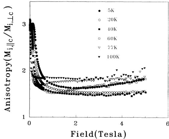
FIG. 5. Anisotropic ratio  $M_{i\parallel c}/M_{i\perp c}$  of initial magnetization as a function of applied magnetic field at 5, 20, 40, 60, 77, and 100 K.
