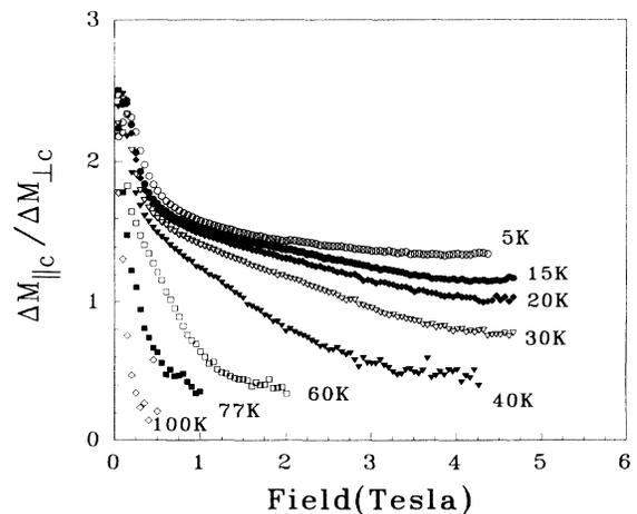
FIG. 7. Anisotropic ratio of the magnetic-flux irreversibility  $\Delta M_{\parallel c}/\Delta M_{\perp c}$  as a function of applied magnetic field at 5, 15, 20, 30, 40, 60, 77, and 100 K.
