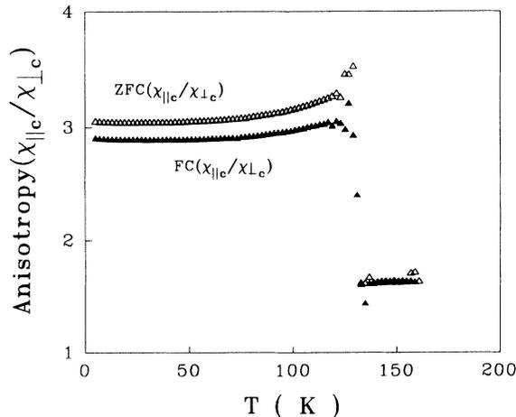
FIG. 3. Temperature dependence of anisotropic ratios of magnetic susceptibility for ZFC and FC samples.
