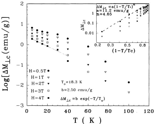
FIG. 9. Temperature dependence of the magnetic-flux irreversibility  $\Delta M_{\perp c}(T)$  at 0.5, 1, 2, 3, and 4 T. Exponential dependence of  $\Delta M_{\perp c}(T)$  below 30 K was observed. [The inset displays the logarithmic plots of  $\Delta M_{\perp c}(T)$  versus  $(1-T/T_c)$  at the fields mentioned above.]
