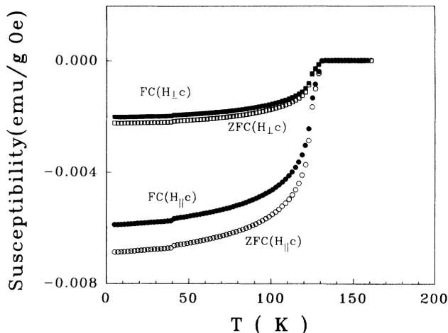
FIG. 2. Temperature dependence of magnetic susceptibility for both the parallel and the perpendicular directions to the *c* axis.
