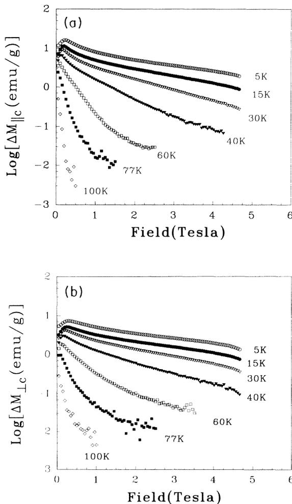
FIG. 6. (a) Magnetic-field dependence of the magnetic-flux irreversibility  $\Delta M_{\parallel c}$  at 5, 15, 30, 40, 60, 77, and 100 K. (b) Magnetic-field dependence of the magnetic-flux irreversibility  $\Delta M_{\perp c}$  at 5, 15, 30, 40, 60, 77, and 100 K.
