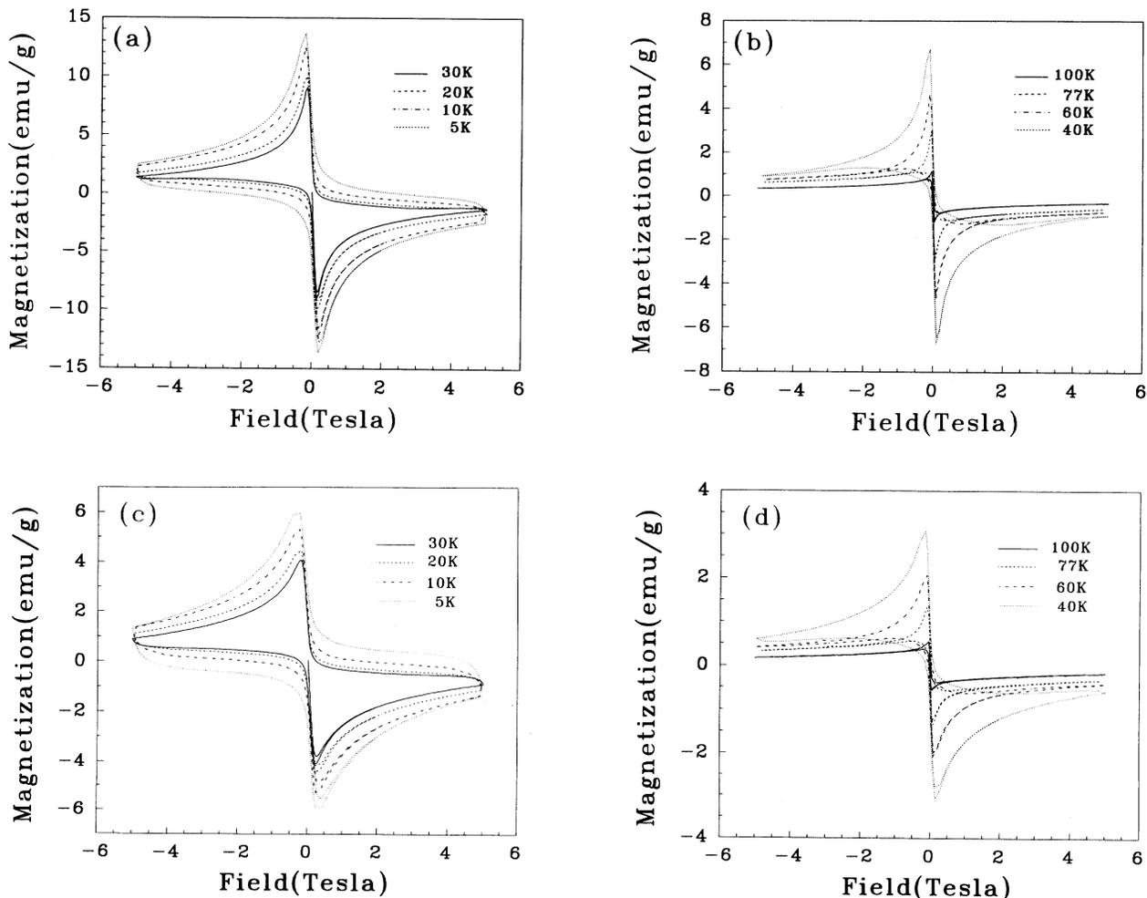
FIG. 4. Magnetization hysteresis loop measured at 5, 10, 20, 30, 40, 60, 77, and 100 K for aligned Hg-1223. (a) and (b) correspond to  $H \parallel c$ , whereas (c) and (d) correspond to  $H \perp c$ .
