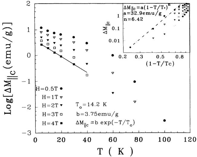
FIG. 8. Temperature dependence of the magnetic-flux irreversibility  $\Delta M_{||c}(T)$  at 0.5, 1, 2, 3, and 4 T. Exponential dependence of  $\Delta M_{||c}(T)$  below 30 K was observed. [The inset displays the logarithmic plots of  $\Delta M_{||c}(T)$  versus  $(1-T/T_c)$  at the fields mentioned above.]
