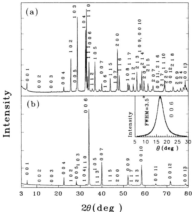
FIG. 1. (a) X-ray diffraction patterns for randomly oriented Hg-1223 powder. (b) XRD pattern of aligned Hg-1223 powders in epoxy. [The inset displays the  $\theta$  rocking curve with FWHM =  $3.5^\circ$  measured at (006).]
