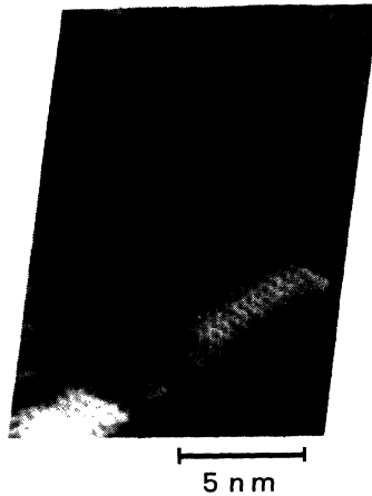
FIG. 3. The STM image of the graphite-covered TaC(111) surface taken at the bias voltage of 2.4 V and the tunneling current of 0.08 nA. The dark area in the lower right represents the lower terrace.
