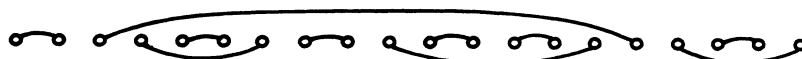
FIG. 2. A schematic of the random-singlet ground state. Each spin forms a singlet pair with another spin indicated by the connecting “bond” lines. Most pair with nearby spins, but pairs with arbitrarily long distances separating the two spins also exist. Note that the bonds do not cross each other.
