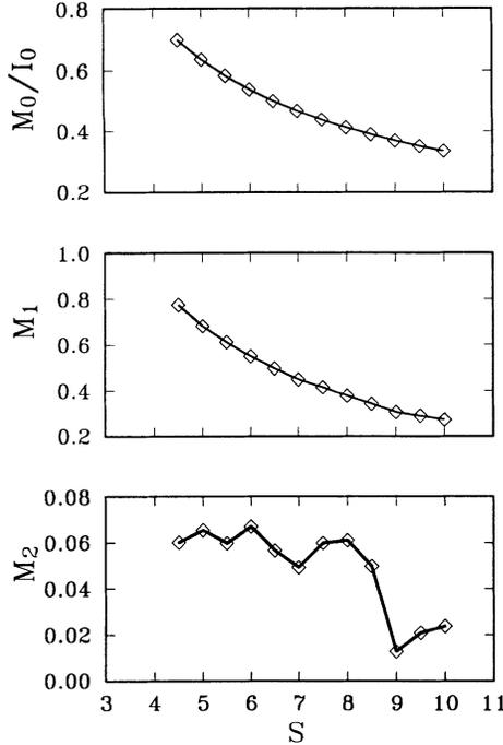
FIG. 18. Integrated intensity ( $M_0$ ), centroid ( $M_1$ ), and linewidth ( $M_2$ ) of the PL spectrum for an  $e-A^0$  system ( $N_e=7$  and  $N_h=1$ ) at  $d=3.0$ .  $M_1$  and  $M_2$  are in units of  $e^2/\epsilon l$ .
