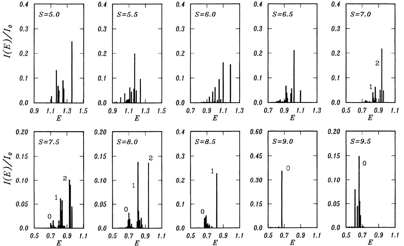
FIG. 4. Photoluminescence spectrum of an  $e$ - $h$  system ( $N_e = 7$  and  $N_h = 1$ ) at  $d = 8.0$  and  $T = 0.005e^2/\epsilon l$  for  $S$  values from 5.0 to 9.5. Energy is in units of  $e^2/\epsilon l$ .  $d$  is in units of the magnetic length  $l$ . The number beside a PL peak indicates the quasielectron process (Fig. 5 below) from which the peak results.
