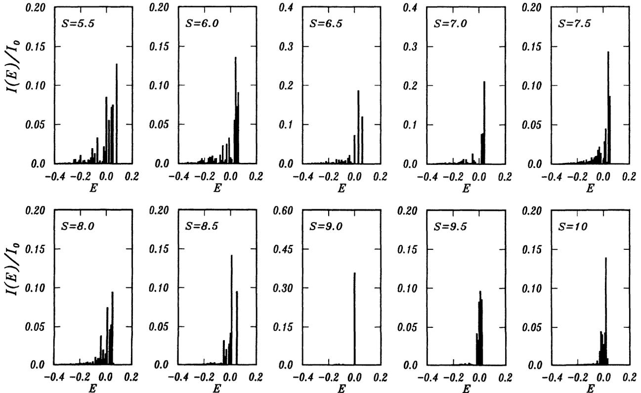
FIG. 16. Photoluminescence spectrum of an  $e-A^0$  system ( $N_e=7$  and  $N_h=1$ ) at  $d=0$  and  $T=0.005e^2/\epsilon l$  for  $S$  values from 5.5 to 10. Energy is in units of  $e^2/\epsilon l$ .
