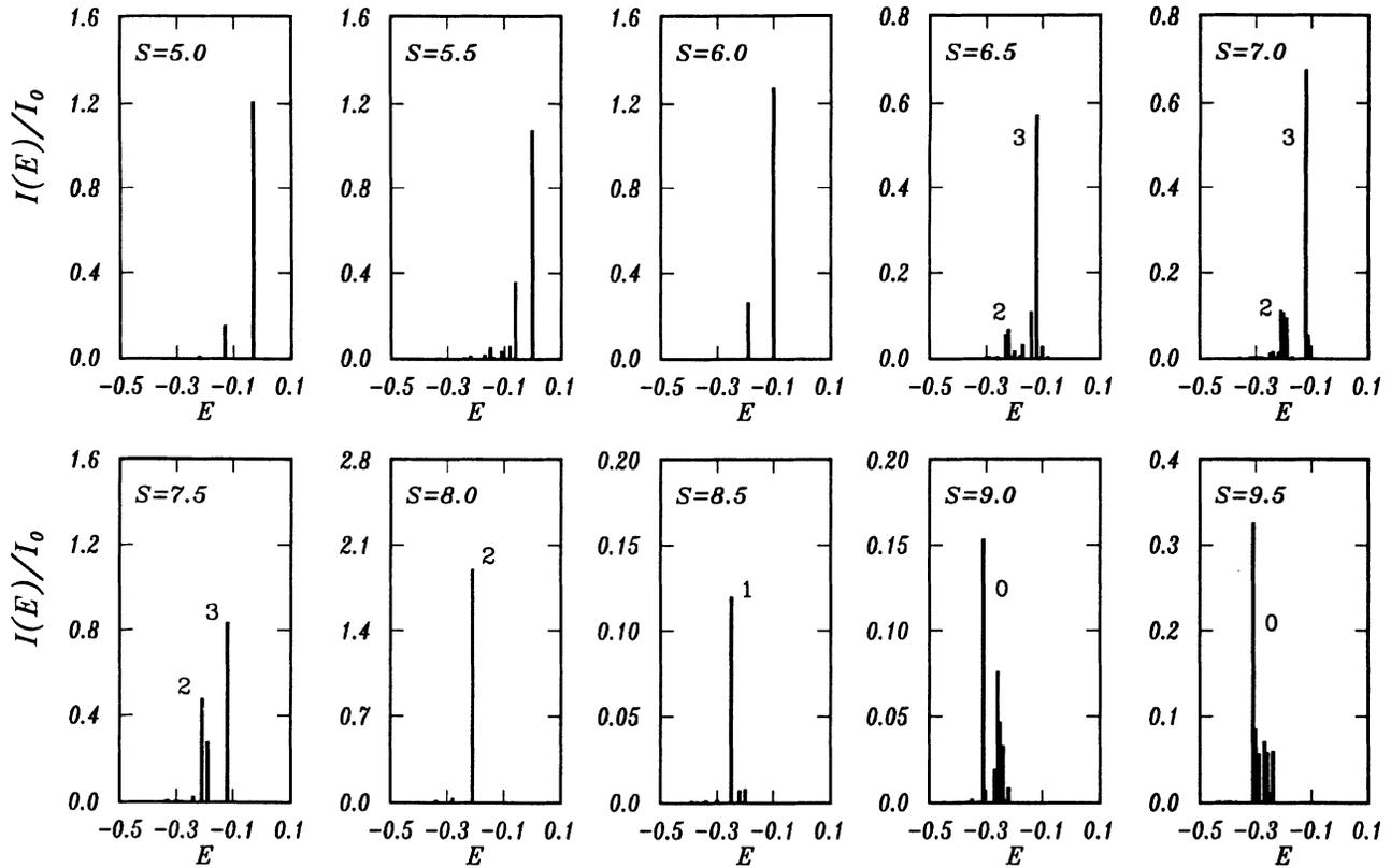
FIG. 9. Photoluminescence spectrum of an  $e$ - $h$  system ( $N_e=7$  and  $N_h=1$ ) at  $d=1.75$  and  $T=0.005e^2/\epsilon l$  for  $S$  values from 5.0 to 9.5. Energy is in units of  $e^2/\epsilon l$ . The number beside a PL peak indicates the quasi-electron process (Fig. 5) from which the peak results.
