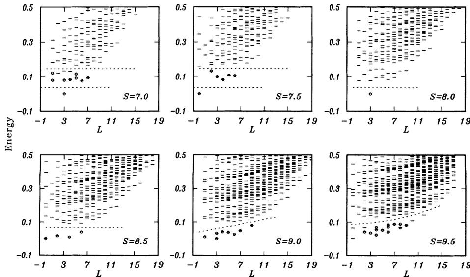
FIG. 10. Energy spectra of a six-electron system. States circled are those to which the optical transitions contribute significantly to the PL spectrum of Fig. 9.
