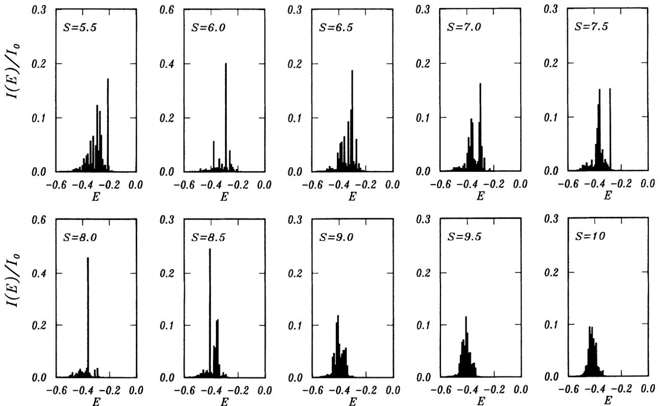
FIG. 14. Photoluminescence spectrum of an  $e-A^+$  system ( $N_e=7$  and  $N_h=1$ ) at  $d=1.3$  and  $T=0.02e^2/\epsilon l$  for  $S$  values from 5.5 to 10. Energy is in units of  $e^2/\epsilon l$ .
