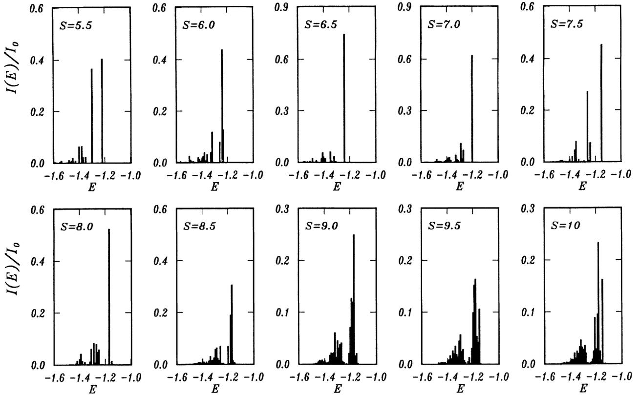
FIG. 12. Photoluminescence spectrum of an  $e-A^+$  system ( $N_e=7$  and  $N_h=1$ ) at  $d=0$  and  $T=0.005e^2/el$  for  $S$  values from 5.5 to 10. Energy is in units of  $e^2/el$ .
