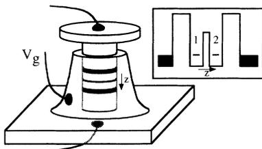
FIG. 1. Proposed experimental setup for a sidewall-gated small-cross-section vertical triple barrier structure. Inset shows the simplified conduction band in the central region in the growth direction. Fermi energy and lateral confinement can be changed with the gate voltage  $V_g$ .
