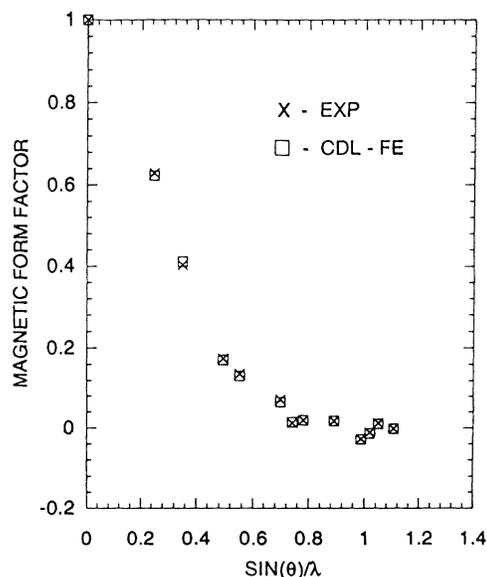
FIG. 3. Comparison of theoretical and experimental form factors normalized to unity at (000) for iron ( $\lambda$  in Å). Theory result based on CLD bands; experimental results from Shull and Yamada (Ref. 13).
