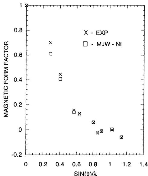
FIG. 2. Comparison of theoretical and experimental form factors normalized to unity at (000) for nickel ( $\lambda$  in Å). Theory result based on MJW local density bands; experimental results from Mook (Ref. 12).
