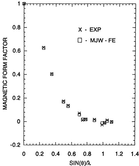
FIG. 4. Comparison of theoretical and experimental form factors normalized to unity at (000) for iron ( $\lambda$  in  $\text{\AA}$ ). Theory result based on MJW local density bands; experimental results from Shull and Yamada (Ref. 13).
