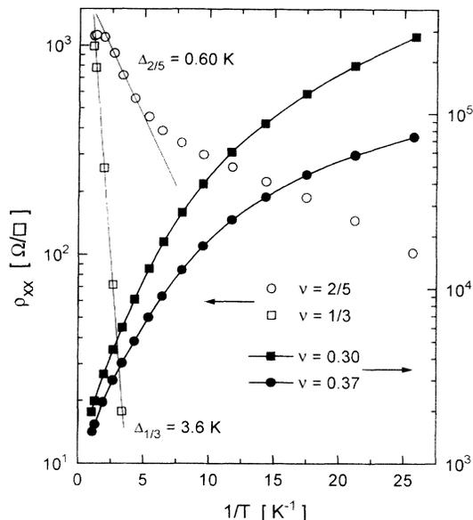
FIG. 3. Temperature dependence of  $\rho_{xx}$  for the reentrant IP at  $\nu = 0.37$  and  $0.30$  (right axis), and for the FQH states at  $\nu = 2/5$  and  $1/3$  (left axis). Lines through the FQH data represent fits to the activated regions, from which the quasiparticle excitation gaps  $\Delta_\nu$  were determined.
