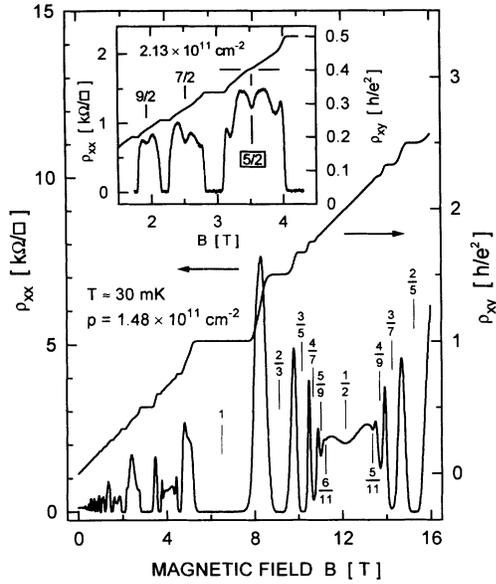
FIG. 1. Main figure:  $\rho_{xx}$  and  $\rho_{xy}$  vs  $B$  for a 2DHS. Filling factors  $\nu$  are marked with vertical lines. Inset: data from the same sample at higher density, where a developing  $\nu = 5/2$  FQH state is observed.
