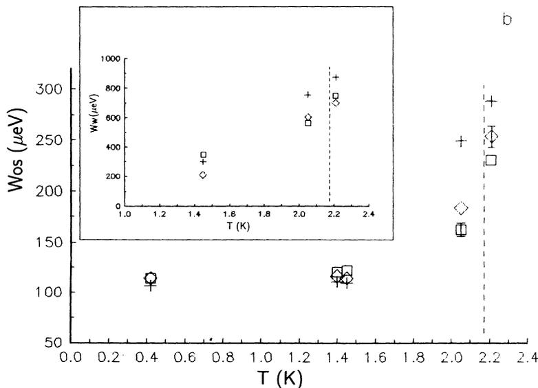
FIG. 11. Temperature dependence of intrinsic widths of peaks. (a)  $q \sim 1 \text{ \AA}^{-1}$ . (n) open circles, (w) closed circles. Resolution is subtracted. The solid curve shows  $W(T)$  [Eq. (9)]. (b) (os) component and (w) component (see inset).  $q = 0.28 \text{ \AA}^{-1}$  squares,  $q = 0.37 \text{ \AA}^{-1}$  diamonds, and  $q = 0.45 \text{ \AA}^{-1}$  pluses. Resolution is not subtracted.
