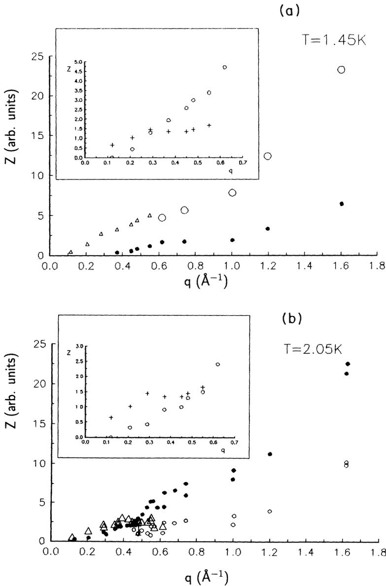
FIG. 6. Wave-vector dependence of the component areas at: (a)  $T = 1.45 \text{ K}$ ; (b)  $T = 2.05 \text{ K}$ ; (c)  $T = 2.21 \text{ K}$ . (*n*) open circles, (*w*) closed circles, and (*os*) triangles. Two-part-decomposition of the (*os*) component [(*os*) component at  $T = 2.21 \text{ K}$ , pluses and (*n*) component, open circles] is shown in the inset. (d) The contribution  $Z(q)$  of the one-phonon excitations to the total scattering  $S(q)$  at  $1.1 \text{ K}$  from Ref. 7.
