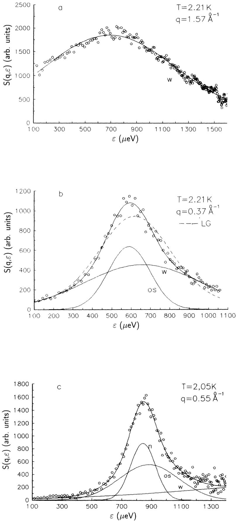
FIG. 3.  $S(q, \epsilon)$  and its decomposition components at various temperatures and wave vectors. For comparison, the single Lorentzian fit (LG) is shown in (b).
