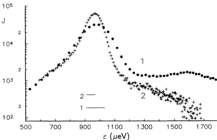
FIG. 2. Comparison of the experimental neutron-scattering spectra of liquid  $^4\text{He}$  at  $q \sim 1.6 \text{ \AA}^{-1}$  for different initial energies. (1)  $T = 1.5$  K and  $E_0 = 3.5$  meV; (2)  $T = 1.45$  K and  $E_0 = 2.08$  meV. Instrumental resolution in the range of peaks are shown by the horizontal lines. Spectra are normalized to the single-particle peak areas.
