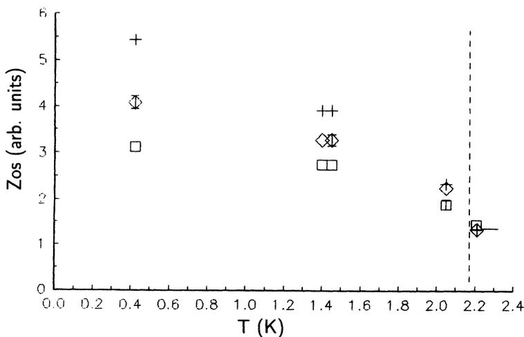
FIG. 9. Temperature dependence of the (*os*)-component areas:  $q = 0.28 \text{ \AA}^{-1}$  squares,  $q = 0.37 \text{ \AA}^{-1}$  diamonds, and  $q = 0.45 \text{ \AA}^{-1}$  pluses.
