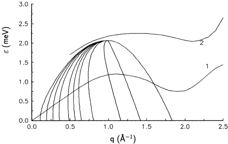
FIG. 1. The phonon-rotor dispersion curve in superfluid helium-4 (1) and multiphonon excitations (2). The kinematics laws at various angles scattering at incident neutron energy  $E_0 = 2.08$  meV are shown [see Eq. (4)].
