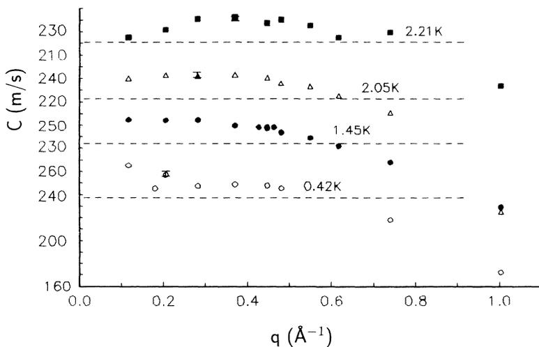
FIG. 12. Velocity of sound at various temperatures for the components (*os*). Liquid-helium first-sound velocity is shown by horizontal dashed lines (Ref. 42).
