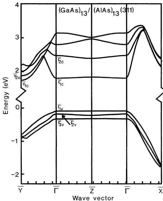
FIG. 1. Electronic band structure of  $(\text{GaAs})_{13}/(\text{AlAs})_{13}$  (311) superlattice along the directions  $(0\bar{1}\bar{1})\bar{\Gamma}-\bar{X}$ ,  $(233)\bar{\Gamma}-\bar{Y}$ , and  $(311)\bar{\Gamma}-\bar{Z}$ .
