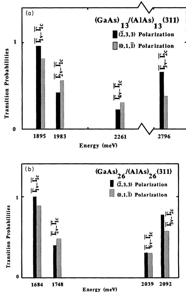
FIG. 3. Transition probabilities (in arbitrary units) between the valence states  $\bar{\Gamma}_{1v}$  and the conduction states  $\bar{\Gamma}_{jc}$  for two  $(\text{GaAs})_N/(\text{AlAs})_N$  (311) superlattices (a)  $N=13$  and (b)  $N=26$  in the two polarization directions  $[-2, 3, 3]$  and  $[0, -1, 1]$ .
