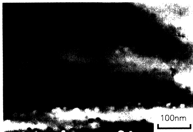
FIG. 2. Bright-field image of the \gamma' phase with a thickness contrast. The \gamma' precipitates have a larger extinction distance than the matrix and are imaged alternately in bright and dark contrast.
