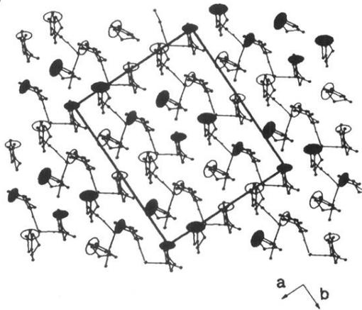
FIG. 6. (a) STM image of a  $(\text{BEDT-TTF})_2\text{Cu}(\text{NCS})_2$  crystal with periodic modulation in charge density ( $V_t=23$  mV,  $I_s=2.7$  nA,  $9\times 9$  nm<sup>2</sup>). (b) Molecular arrangement of  $\alpha$ - $(\text{BEDT-TTF})_2\text{Cu}(\text{NCS})_2$ . A  $2\times 2$  unit cell with modulated charge density on the BEDT-TTF molecules is indicated by hatched and open ellipses.
