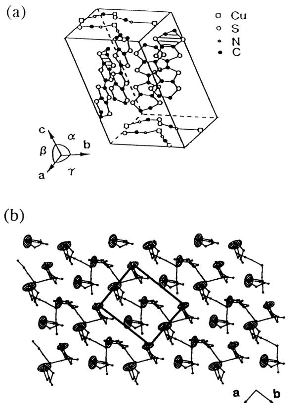
FIG. 3. (a) Crystal structure of  $\alpha$ -(BEDT-TTF)<sub>2</sub>Cu(NCS)<sub>2</sub>. (b) Molecular arrangement of the  $\alpha$ -(BEDT-TTF)<sub>2</sub>Cu(NCS)<sub>2</sub> crystal projected on the crystal  $a$ - $b$  plane ( $\square$ , Cu;  $\circ$ , S;  $\bullet$ , C;  $\circ$ , N).
