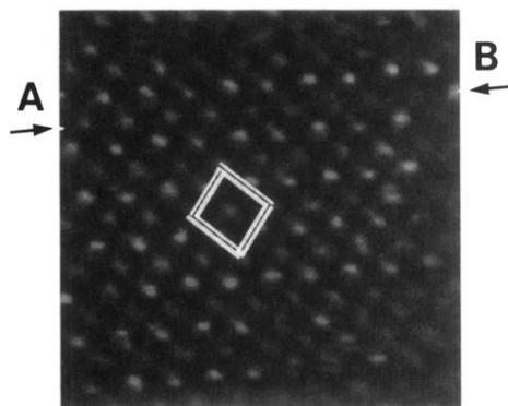
FIG. 2. STM image of a  $(\text{BEDT-TTF})_2\text{Cu}(\text{NCS})_2$  crystal surface ( $V_t = -22$  mV,  $I_s = 2.8$  nA,  $6.5 \times 6.5 \text{ nm}^2$ ).
