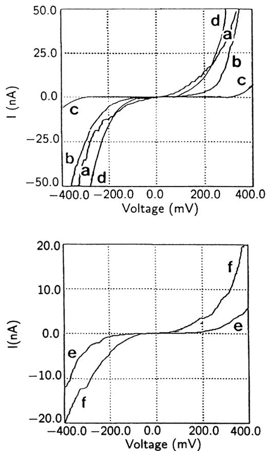
FIG. 5. Series of  $I$ - $V$  curves measured at curves  $a$ , 277;  $b$ , 175;  $c$ , 27.7;  $d$ , 7.8; and  $e$ , 78 K.  $I$ - $V$  curve  $f$ , measured at 78 K under soft contact of the tip with the sample surface.
