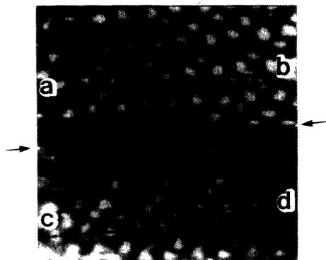
FIG. 4. STM image of a domain structure in a  $(\text{BEDT-TTF})_2\text{Cu}(\text{NCS})_2$  crystal surface. Domain boundary is indicated by arrows.
