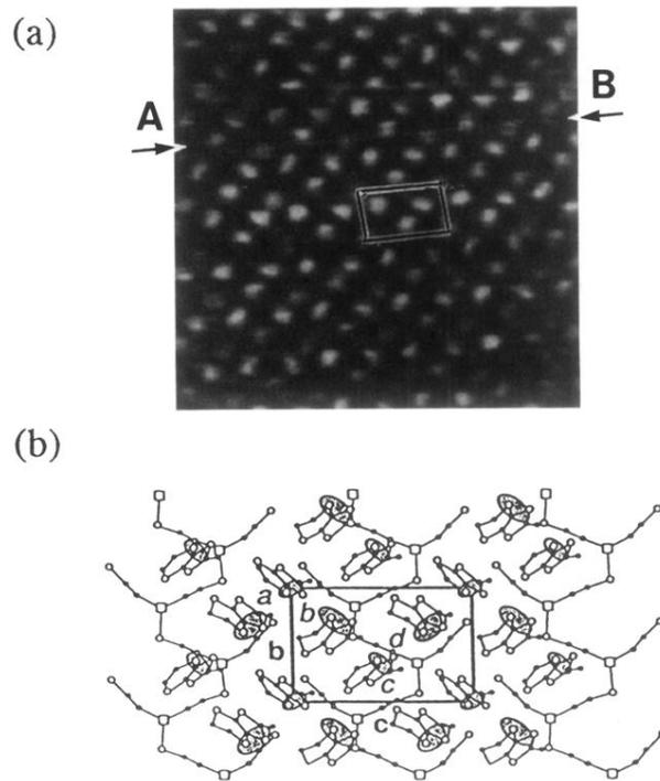
FIG. 1. (a) STM image of a  $(\text{BEDT-TTF})_2\text{Cu}(\text{NCS})_2$  crystal ( $V_t = -22$  mV,  $I_s = 2.8$  nA,  $6.5 \times 6.5$  nm<sup>2</sup>). (b) Molecular arrangement of the  $(\text{BEDT-TTF})_2\text{Cu}(\text{NCS})_2$  crystal projected on the crystal  $b$ - $c$  plane ( $\square$ , Cu;  $\circ$ , S;  $\bullet$ , C;  $\circ$ , N) (Ref. 4).
