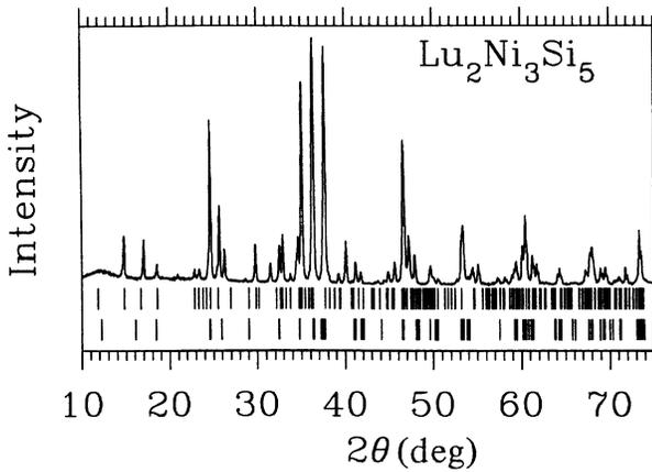
FIG. 1. Room-temperature powder-x-ray-diffraction pattern of  $\text{Lu}_2\text{Ni}_3\text{Si}_5$ . The upper bars correspond to the positions of XRD peaks permitted by the space group  $C2/c$ , while the lower bars correspond to the positions permitted by space group  $Ibam$ .
