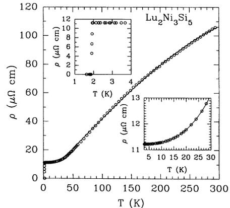
FIG. 3. Resistivity of  $\text{Lu}_2\text{Ni}_3\text{Si}_5$  from 1.5 to 300 K. The solid line is a fit to Eq. (2). The insets show the superconducting transition and a  $T^3$  dependence of  $\rho(T)$  at low temperatures. Solid lines are fit to the models (see text).
