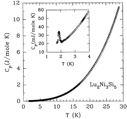
FIG. 4. Temperature dependence of specific heat of  $\text{Lu}_2\text{Ni}_3\text{Si}_5$  from 1.7 to 30 K. The inset shows an expanded plot at low temperatures. The solid line is a fit to Eq. (3).
