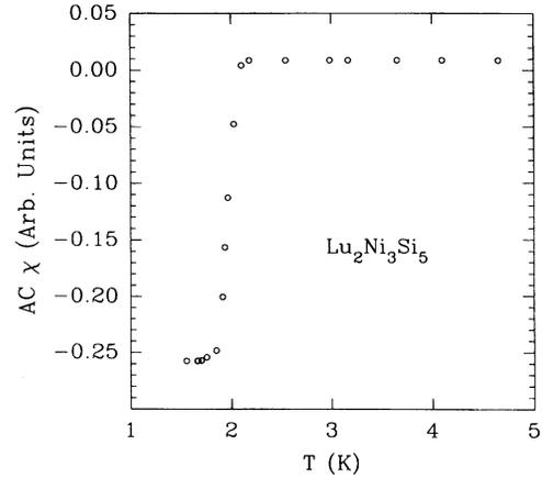
FIG. 2. ac susceptibility of  $\text{Lu}_2\text{Ni}_3\text{Si}_5$  from 1.5 to 5 K.
