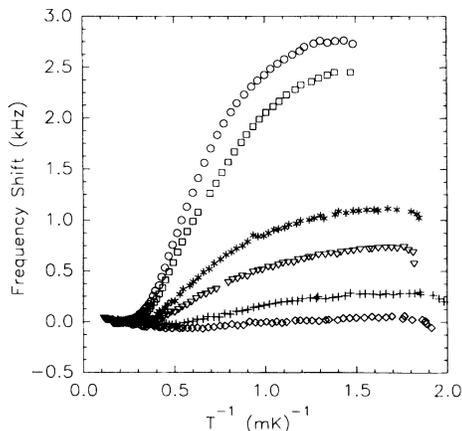
FIG. 3. Frequency shift of the maximum of the NMR line shape as a function of temperature at various coverages. ( $\diamond$ )  $0.193 \text{ \AA}^{-2}$ , ( $+$ )  $0.196 \text{ \AA}^{-2}$ , ( $\nabla$ )  $0.198 \text{ \AA}^{-2}$ , ( $*$ )  $0.200 \text{ \AA}^{-2}$ , ( $\square$ )  $0.211 \text{ \AA}^{-2}$ , ( $\circ$ )  $0.222 \text{ \AA}^{-2}$ . Data for coverages  $0.185$  and  $0.188 \text{ \AA}^{-2}$  show zero shift and are not plotted for clarity.
