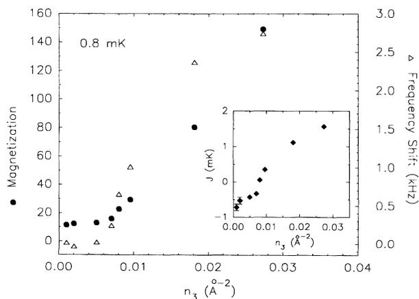
FIG. 5. Isotherms (0.8 mK) of magnetization, frequency shift, and (inset) exchange parameter as a function of third layer fluid coverage.
