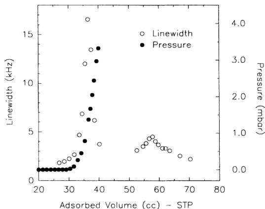
FIG. 1. Isotherms of NMR linewidth (10 mK) and vapor pressure (4.2 K). Second layer promotion occurs at  $36.2 \pm 0.3$  STP  $\text{cm}^3$ .
