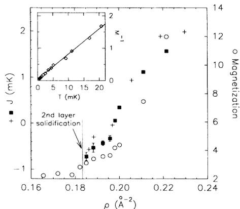
FIG. 2. Isotherms of magnetization at 3.2 mK ( $\circ$ ), and exchange parameter  $J$  for pure  $^3\text{He}$  films ( $\blacksquare$ ). Also shown are data of Ref. 6 for  $^4\text{He}$  preplated graphite ( $+$ ). Inset shows fit to magnetization at  $0.185 \text{ \AA}^{-2}$ .
