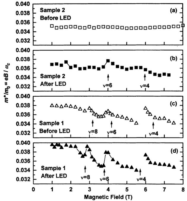
FIG. 3. Electron-hole pair density dependence of CR mass oscillation at 4.2 K. The lower panel for each sample [(b) and (d)] shows data for a higher pair density obtained by illumination with a red LED.
