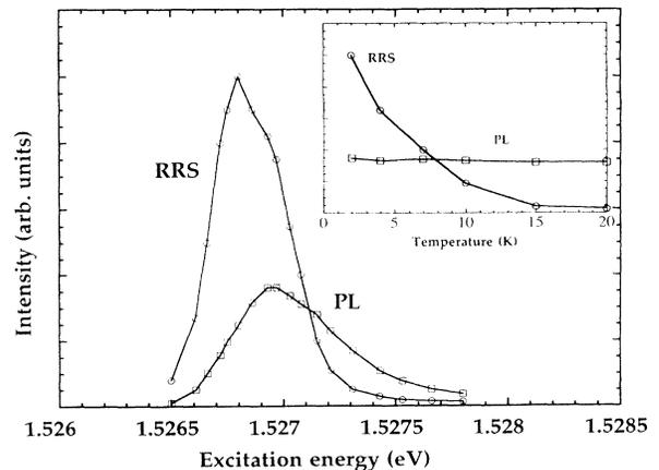
FIG. 2. Intensities of RRS (dots) and PL (squares) as a function of the excitation energy in the case of the 180-Å QW; the lines are only guides for the eye. In the inset the temperature dependence of the RRS and PL signals is reported.
