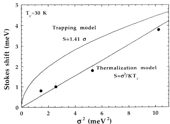
FIG. 9. Measured Stokes shifts at  $T_C = 30$  K as a function of the standard deviation  $\sigma$  obtained from a Gaussian fit of the PLE excitonic lines. The straight line demonstrates the quadratic dependence of the SS on  $\sigma$ .
