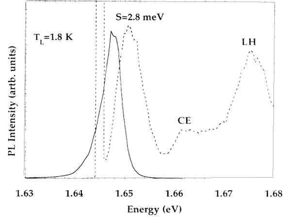
FIG. 6. Comparison between the PL (full line) and PLE (dashed line) spectra for the 40-Å QW at  $T_L = 1.8$  K. We find a SS of 2.8 meV. Note that the continuum edge (CE) and the light-hole (LH) exciton recombination are resolved in the PLE spectrum.
