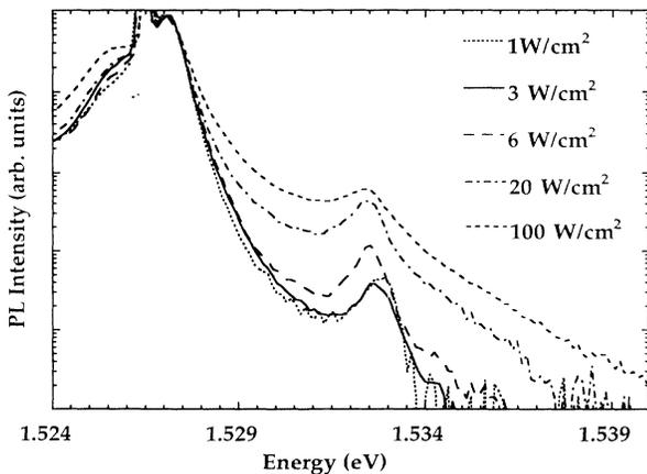
FIG. 5. PL spectra of the 180-Å QW as a function of the excitation intensity for resonant excitation at  $T_L = 10$  K.
