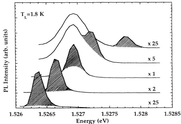
FIG. 1. PL spectra of the 180-Å QW at  $T_L = 1.8$  K for different excitation energies showing a resonant enhancement of the RS (hatched areas) when the excitation is tuned across the HH exciton band. The relative scale factors of the PL spectra are also given in the figure.
