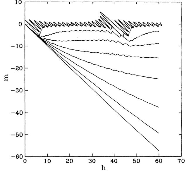
FIG. 1. Initial magnetization curves  $m(h)$  for the studied Josephson-junction array. The  $h$  steps are 0.2. From the bottom curve upwards, the average field-sweeping rate  $(dh/dt^*)_{\text{av}} = 20, 2, 0.5, 0.2, 0.1, 0.05, 0.02$ , and 0.002. The upper oscillatory curve is static.
