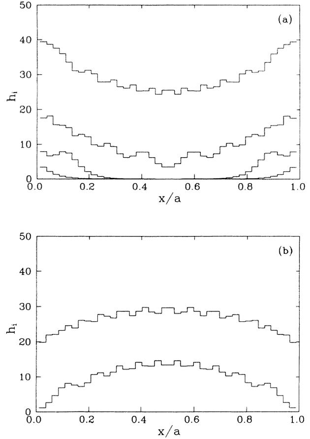
FIG. 3. The internal field profiles for the magnetic states on the curve in Fig. 2. (a) The curves from down to up correspond to  $h = 5, 10, 20$ , and  $40$  on the initial  $m(h)$  curve. (b) The curves from up to down are for  $h = 20$  and  $0$  on the reverse  $m(h)$  curve.
