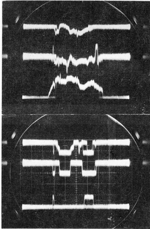
FIG. 5. Induced voltage (across bad junction) vs time (synchronized to the sweep mode of the microwave radiation shown in the upper trace of Fig. 3).  $P_{\text{rms}} = 5 \times 10^{-4}$  W. Vertical scale,  $20 \mu\text{V}/\text{div}$ . Magnetic field from top to bottom traces 0, 0.1, 0.2, 0.5, 0.6, 0.8 kG. All traces are superposition of eight complete cycles.
