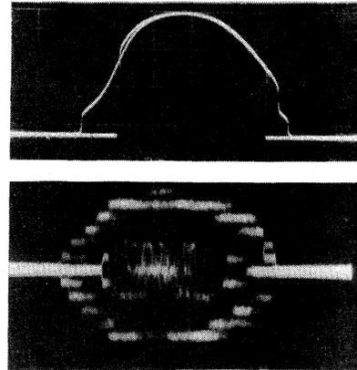
FIG. 3. Upper trace: power spectrum of the klystron output.  $P_{\text{rms}}=1.2 \times 10^{-4}$  W. Horizontal sweep rate is  $80 \text{ Hz}$ , the central frequency  $10 \text{ GHz}$ , and the signal width  $65 \text{ MHz}$ . Lower trace: induced quantum voltage vs frequency and time (synchronized to the horizontal of the upper trace). Vertical,  $50 \mu\text{V}/\text{div}$  (center is shifted slightly to the left).
