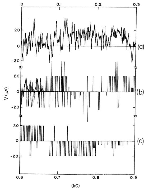
FIG. 6. Induced voltage (across bad junction) vs magnetic field (perpendicular to Pb films). Horizontal axes are (a) 0–0.3 kG; (b) 0.3–0.6 kG; (c) 0.6–0.9 kG. Both microwave power and frequency are fixed, where  $P = 3 \times 10^{-4}$  W and  $\nu = 10$  GHz.
