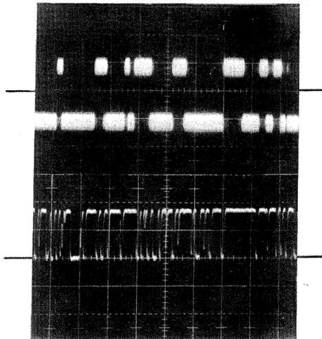
FIG. 2. Induced dc voltages across a Pb—Pb oxide—Pb junction at  $T=1.4$  K and  $H=0$ . Here  $\nu=10$  GHz. Upper trace: vertical,  $20 \mu\text{V}/\text{div}$ ; horizontal,  $0.2 \text{ sec}/\text{div}$ ; microwave power,  $-20 \text{ dBm}$ ,  $n=1$  and  $-1$ . Lower trace: vertical,  $0.1 \text{ mV}/\text{div}$ ; horizontal,  $0.5 \text{ m sec}/\text{div}$ ; microwave power,  $-9 \text{ dBm}$ ,  $n=8$  and  $0$ .
