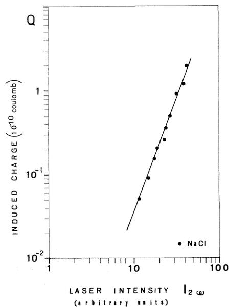
FIG. 4. Three-photon conductivity in NaCl.
