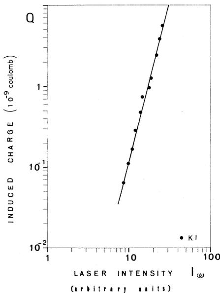
FIG. 1. Four-photon conductivity in KI.
