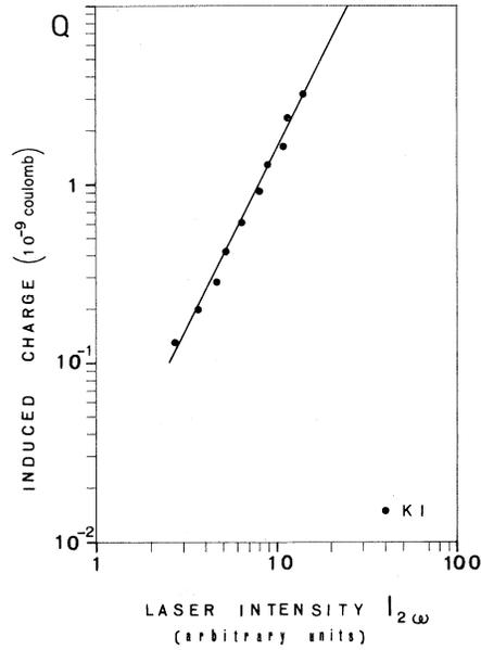
FIG. 2. Two-photon conductivity in KI.
