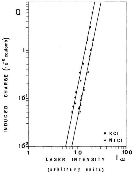
FIG. 3. Five-photon conductivity in KCl and NaCl.
