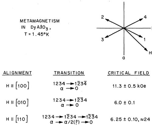
FIG. 1. Four-sublattice model of the magnetic structure (Ref. 9) in  $\text{DyAlO}_3$  and description of the metamagnetic behavior (Refs. 4 and 5) for magnetic fields  $\vec{H}$  applied in the (001) plane. The four vectors describing the magnetization on the sublattices make a constant angle of  $33^\circ \pm 2^\circ$  with the  $b$  axis of the crystal (Ref. 9).
