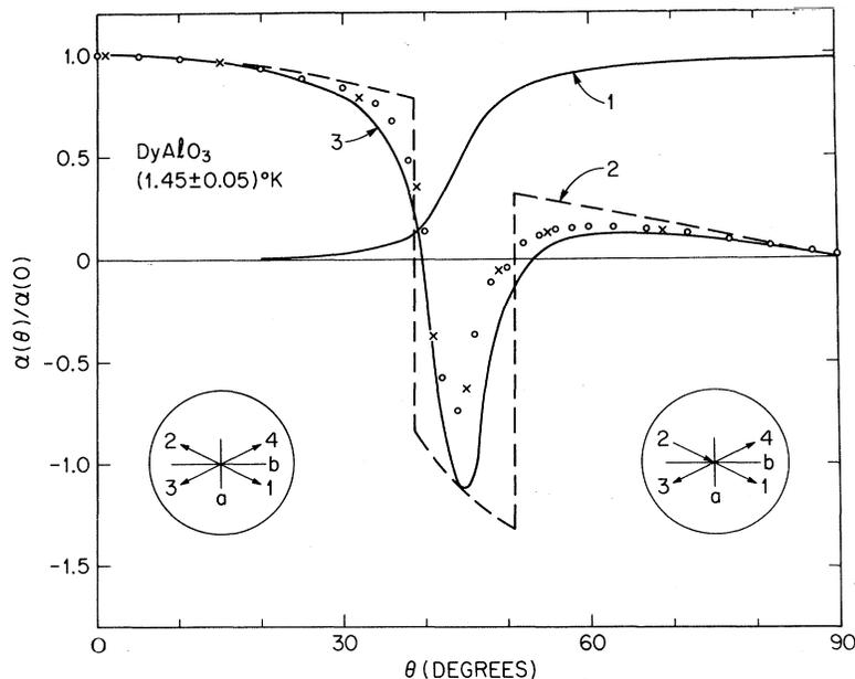
FIG. 4. ME data for rotation into the [110] direction in  $\text{DyAlO}_3$ , with  $H_{dc} = 10$  kOe. The circular points are for increasing  $\theta$  and the x-shaped points are for decreasing  $\theta$ . The insets show the arrangement of the four sublattices at low  $\theta$  and at high  $\theta$  in  $H_{dc} = 10$  kOe. The solid curve No. 1 is the normalized magnetization calculated from the data in Ref. 5. The theoretical curves Nos. 2 and 3 are described in the text.
