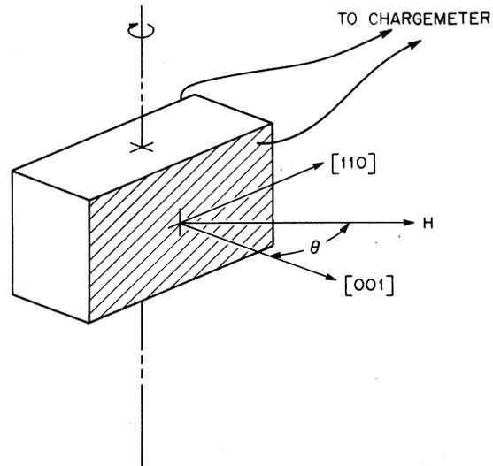
FIG. 2. Experimental arrangement for studying the effect of metamagnetic transitions on the ME signal in  $\text{DyAlO}_3$ . The orientation of the crystal is appropriate to the experiment described in Fig. 4 below.
