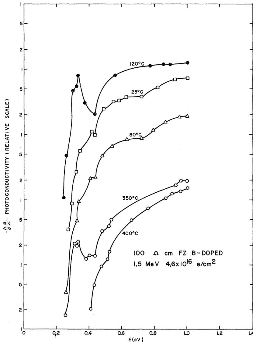
FIG. 6. Isochronal annealing of boron-doped 100- $\Omega$  cm FZ silicon irradiated with  $4.6 \times 10^{16} e/cm^2$  at 1.5 MeV. Experimental error is less than the circle points.
