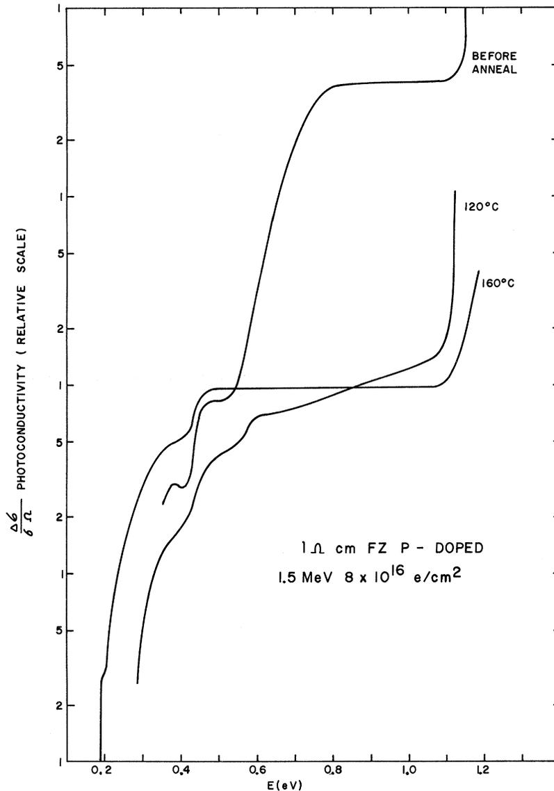
FIG. 10. Isochronal annealing of the  $E_c - 0.54$ -eV energy level.
