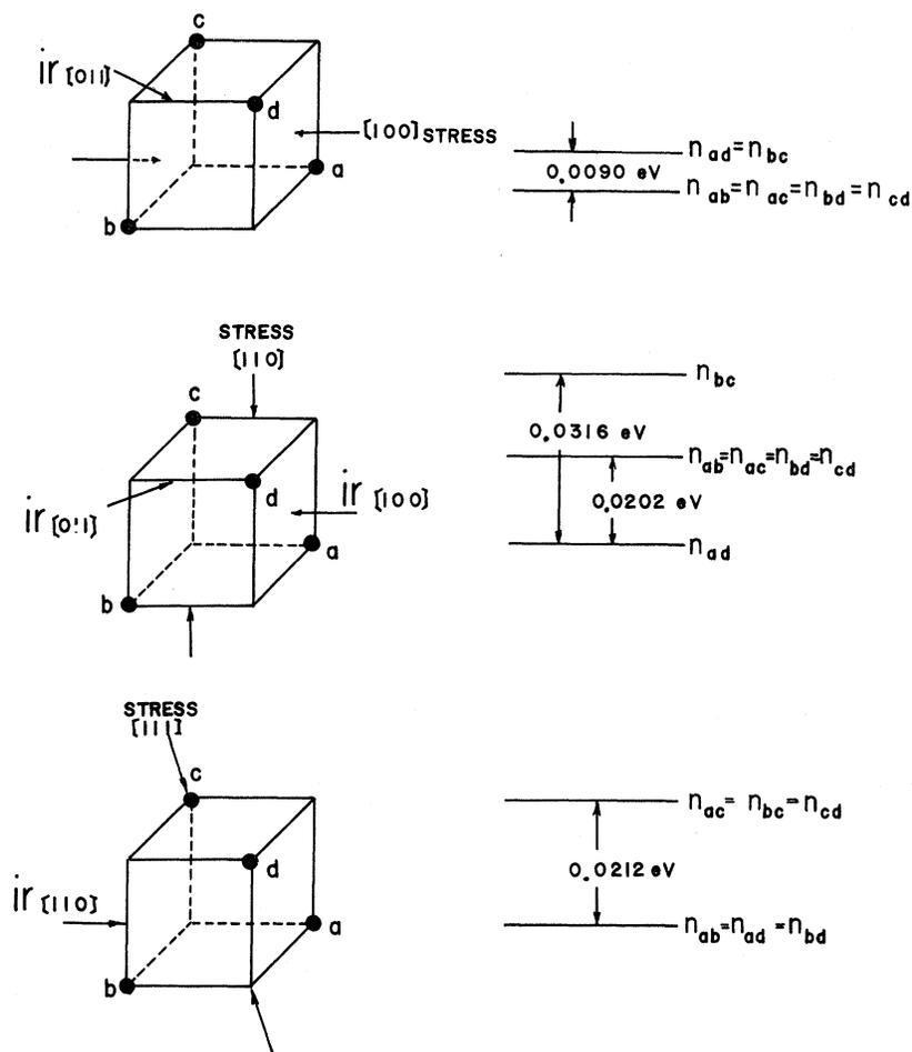
FIG. 12. Nonequivalent-defect-reorientation result by room-temperature stress along three principal crystal axes for the A-center defect.
