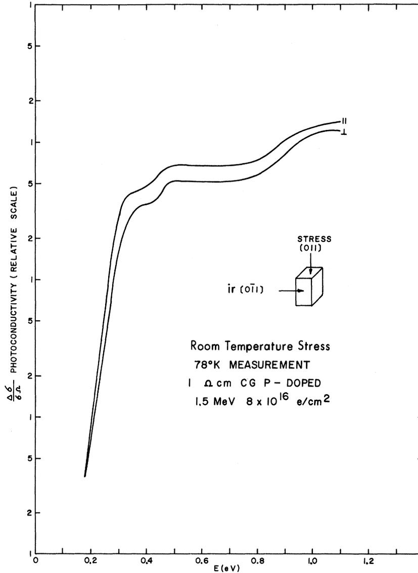
FIG. 11. Dichroism after stress of  $2050 \text{ kg/cm}^2$  at room temperature exhibited by  $1\text{-}\Omega \text{ cm}$  phosphorus-doped CG silicon irradiated with  $8 \times 10^{16} \text{ e/cm}^2$  at  $1.5 \text{ MeV}$ . Experimental error given in text.
