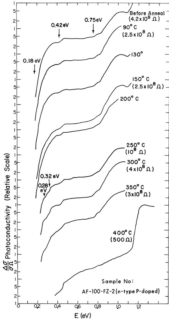
FIG. 4. Isochronal annealing of phosphorus-doped 100-Ω cm FZ silicon irradiated with  $1.6 \times 10^{15}$   $e/\text{cm}^2$  at 1.5 MeV. Experimental error as in Fig. 3. Radiation source: 1.5-MeV electrons  $1.6 \times 10^{15}$   $e/\text{cm}^2$ ; measuring temperature: 78°K; initial resistivity: 100 Ω cm; initial resistance: 420 Ω (78°K).
