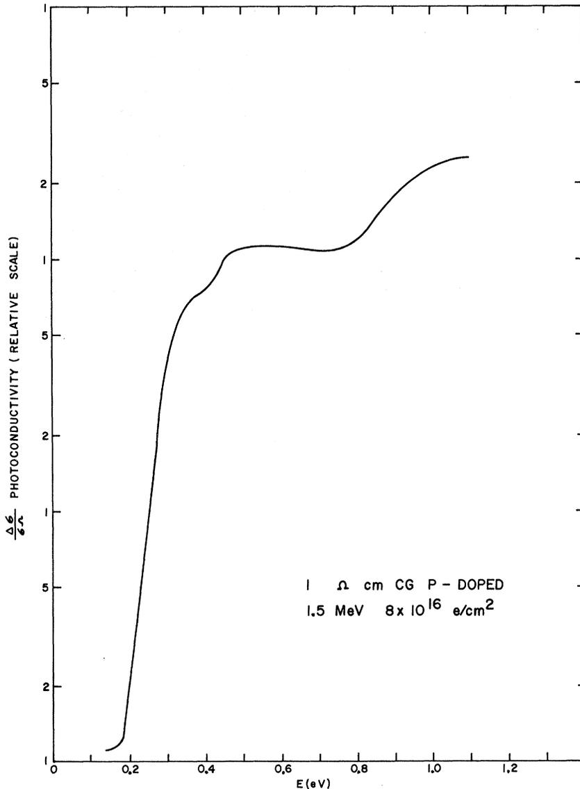
FIG. 7. Photoconductivity spectrum of 1-Ω cm phosphorus-doped CG silicon irradiated with  $8 \times 10^{16}$  e/cm<sup>2</sup> at 1.5 MeV. Experimental error as in Fig. 3.
