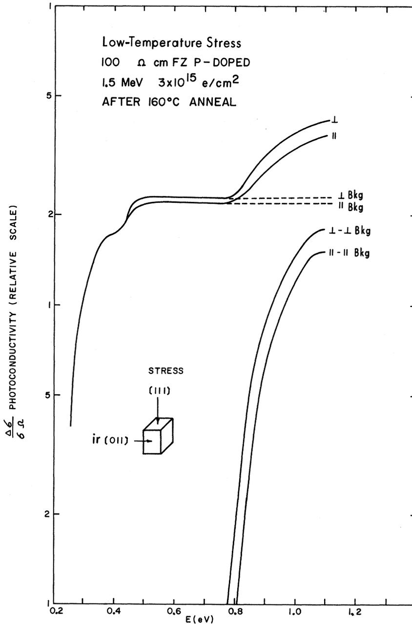
FIG. 5. Dichroism after stress of 2050 kg/cm<sup>2</sup> at 78°K exhibited by 100- $\Omega$  cm phosphorus-doped FZ silicon irradiated with  $3 \times 10^{15}$  e/cm<sup>2</sup> at 1.5 MeV. The sample was annealed to 160°C for 15 min before the stress was applied. The  $\perp$  and  $\parallel$  denote the photoconductivity signal with the incident light polarized with  $\vec{E}$  perpendicular to the stress direction and with  $\vec{E}$  parallel to the stress direction, respectively.
