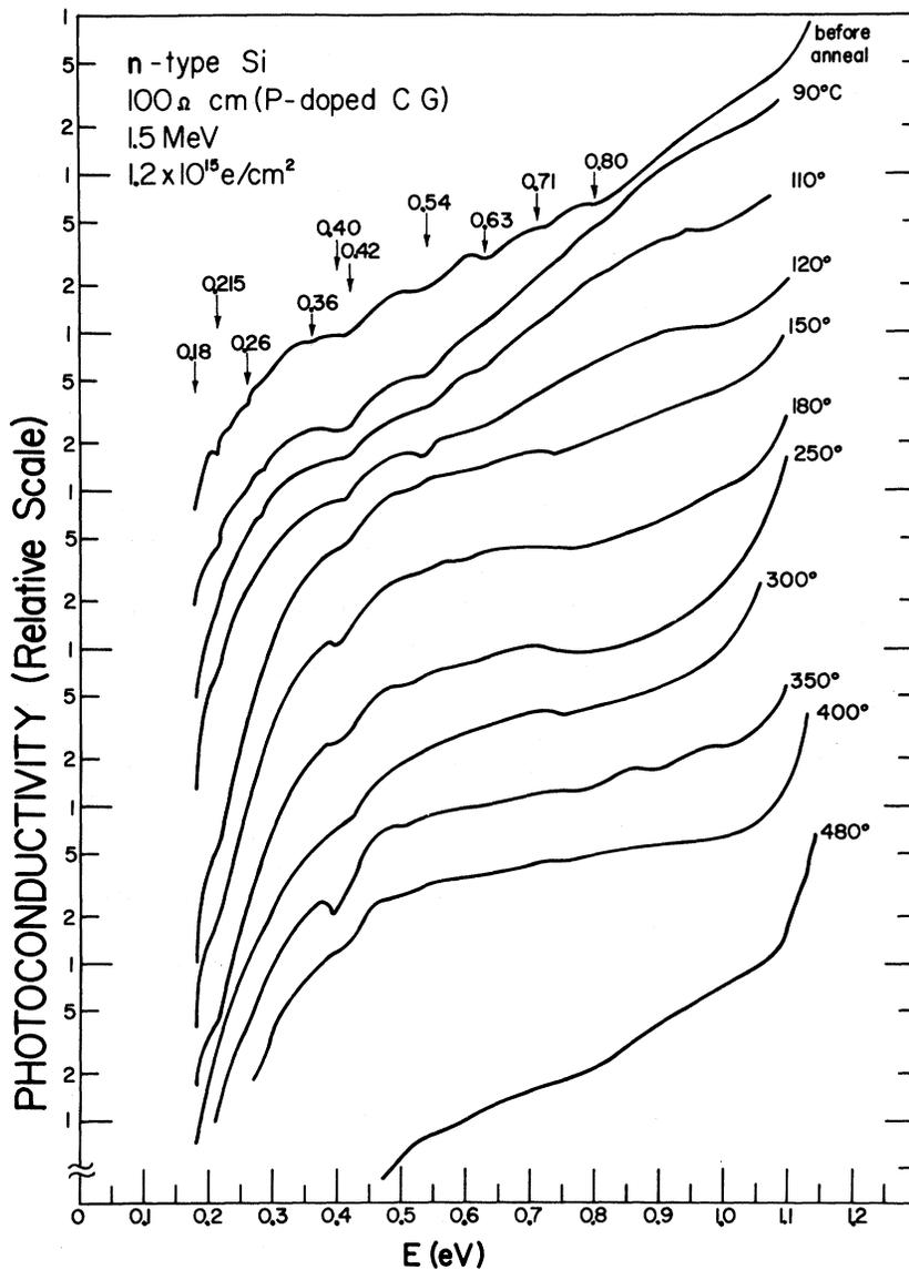
FIG. 9. Isochronal annealing of phosphorus-doped 100- $\Omega$  cm CG silicon irradiated with  $1.2 \times 10^{15}$   $e/cm^2$  at 1.5 MeV. Experimental error as in Fig. 3.
