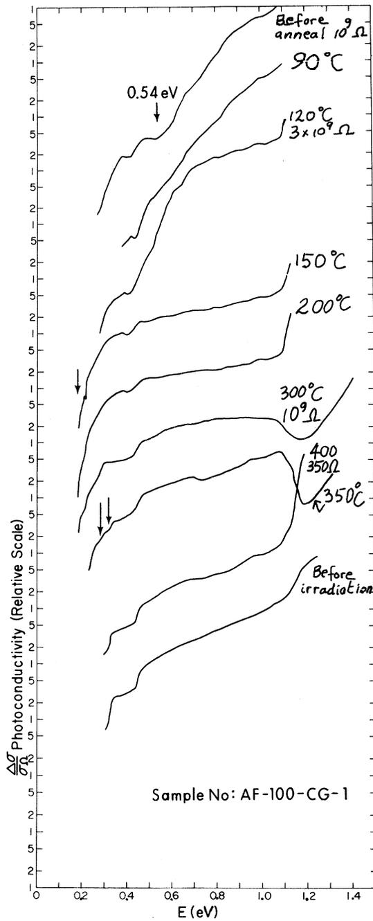
FIG. 8. Isochronal annealing of phosphorus-doped 100- $\Omega$  cm CG silicon irradiated with  $10^3$  rad of  $^{60}\text{Co}$   $\gamma$  rays. Experimental error as in Fig. 3. Measuring temperature: 78°K; initial resistivity: 100  $\Omega$  cm; initial resistance: 380  $\Omega$  (78°K).
