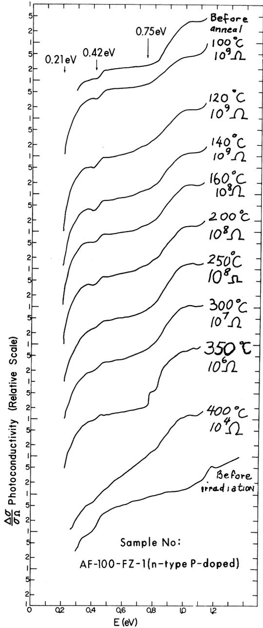
FIG. 3. Isochronal annealing of phosphorus-doped 100-Ω cm FZ silicon irradiated with  $10^8$  rad of  $^{60}\text{Co}$   $\gamma$  rays. Experimental errors are within width of line drawn through points. Radiation source:  $\text{Co}^{60}$   $\gamma$  radiation  $10^8$  rad; measuring temperature: 78°K; initial resistivity: 100 Ω cm; initial resistance: 130 Ω (78°K).
