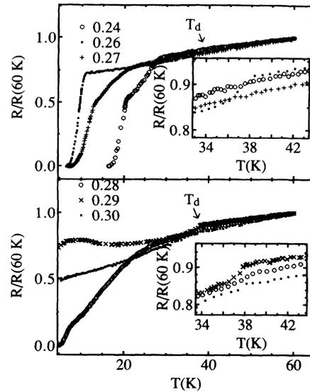
FIG. 3. Resistance versus temperature for six different values of  $x$  in the system  $La_{2-x}Sr_xCuO_4$ .
