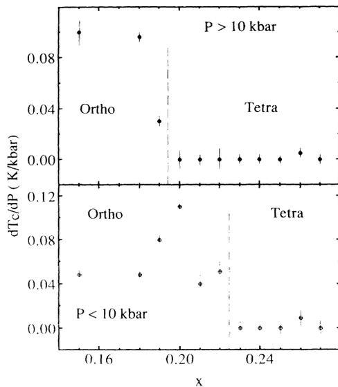
FIG. 2. Variation with  $x$  of the pressure dependence of  $T_c$  for  $P > 10$  kbar and  $P < 10$  kbar in the system  $\text{La}_{2-x}\text{Sr}_x\text{CuO}_4$ .
