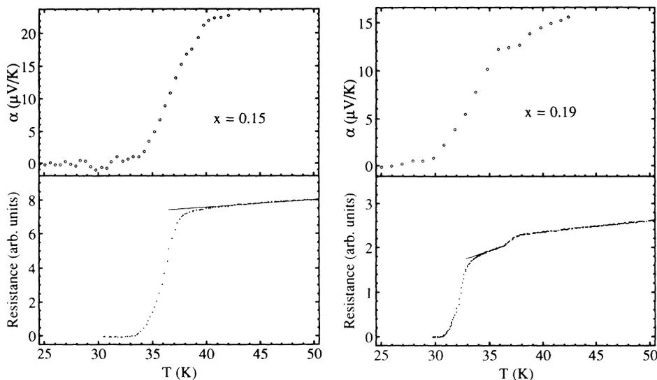
FIG. 4. Temperature variation of Seebeck coefficient  $\alpha$  and resistance  $R$  for samples  $x=0.15$  and  $x=0.19$  of  $\text{La}_{2-x}\text{Sr}_x\text{CuO}_4$ .
