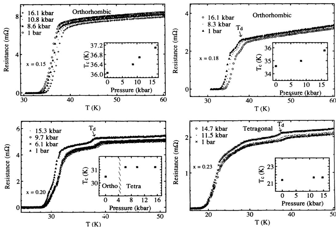
FIG. 1. Temperature dependence of the resistance of  $\text{La}_{2-x}\text{Sr}_x\text{CuO}_4$  pellets under different hydrostatic pressures. Insets: Pressure dependence of  $T_c$ .
