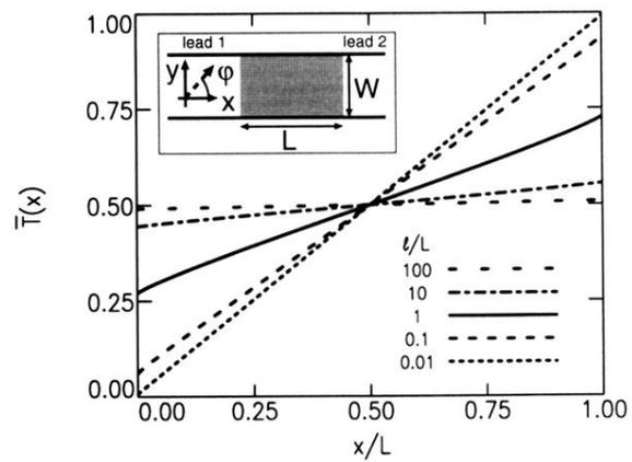
FIG. 1. The conditional transmission probability  $\bar{T}(x)$  as a function of the position along the wire, for various  $\ell/L$ . The inset shows schematically the wire and its coordinates.
