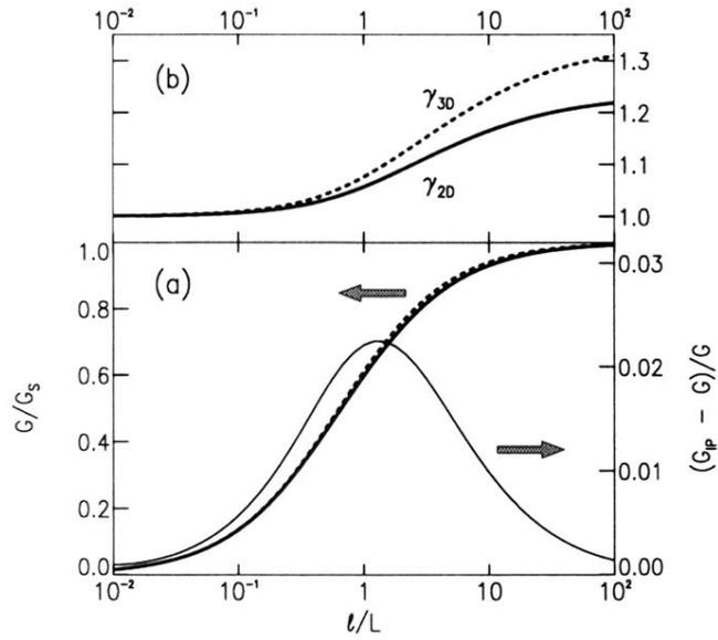
FIG. 2. (a) The conductance [normalized by the Sharvin conductance (2)] plotted against the ratio  $l/L$ . The solid line is from the numerical solution of Eq. (9), the dotted line is  $G_{IP}$  according to the interpolation formula (12). The thin solid line shows the relative error of the interpolation formula. It remains below 2.5%. (b) The dependence on  $l/L$  of the factor  $\gamma_{2D}$  in Eq. (13) (solid line) and  $\gamma_{3D}$  in Eq. (16) (dotted line).
