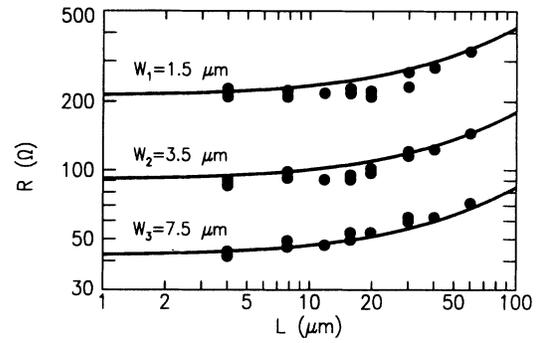
FIG. 3. Comparison between the experimental resistance data of Tarucha *et al.* (Ref. 4) (dots) and the results of our theory (curves). There are no adjustable parameters.
