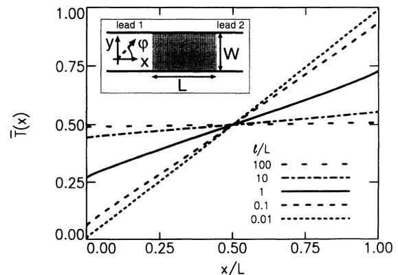
FIG. 1. The conditional transmission probability  $\bar{T}(x)$  as a function of the position along the wire, for various  $\ell/L$ . The inset shows schematically the wire and its coordinates.
