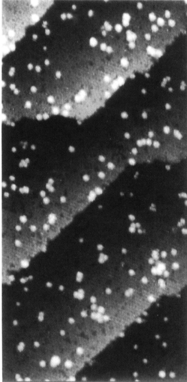
FIG. 5. A STM image measured on the sample surface shown in Fig. 1 following an annealing to 600 °C.
