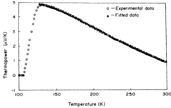
FIG. 2. TEP versus temperature behavior of Bi 2:2:2:3 system.
