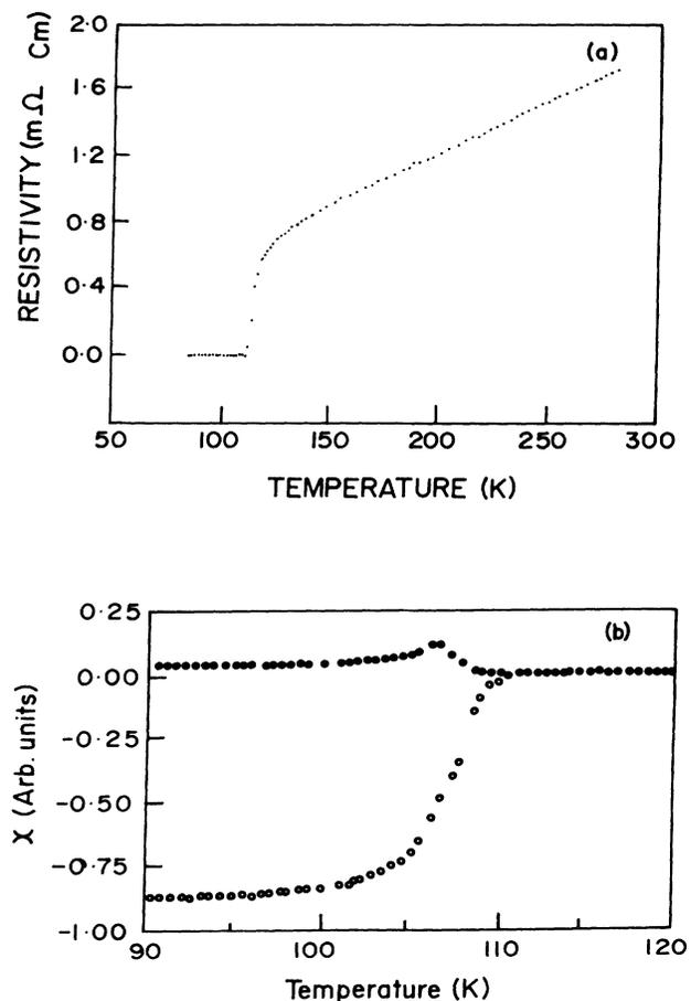
FIG. 1. (a) Resistance versus temperature behavior of  $\text{Bi}_{2:2:2:3}$  system. (b) Ac susceptibility versus temperature behavior of  $\text{Bi}_{2:2:2:3}$  system.
