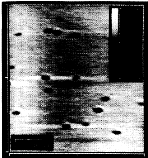
FIG. 1. Continuous contact mode SFM image of single-crystal L -valine irradiated at normal incidence by 78.2-MeV ^{127}\text{I} ions. Some distortion due to tip-surface interactions is apparent.
