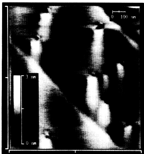
FIG. 2. Continuous contact mode SFM image of single-crystal L -valine irradiated at a 79^\circ grazing angle of incidence. The tail is smooth as evidenced by the preserved step edge seen crossing one of the tails.
