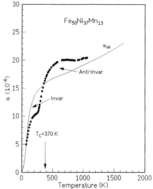
FIG. 7.  $\alpha(T)$  of a FM ground-state Fe<sub>50</sub>Ni<sub>37</sub>Mn<sub>13</sub> sample with a Curie temperature  $T_C = 370$  K. This particular alloy exhibits the Invar effect below  $T_C$  and the anti-Invar effect above it.
