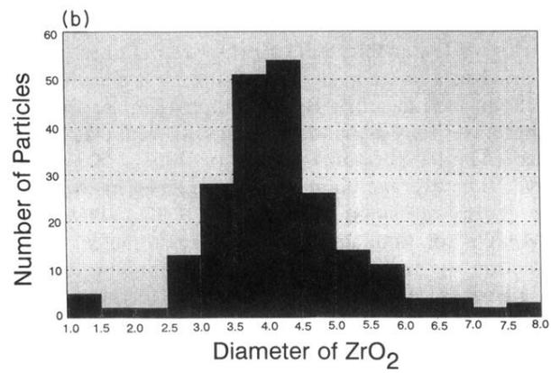
FIG. 1. (a) TEM micrograph of 5-nm diameter ZrO<sub>2</sub> nano-clusters. (b) The distribution of the diameters of the ZrO<sub>2</sub> nano-clusters.
