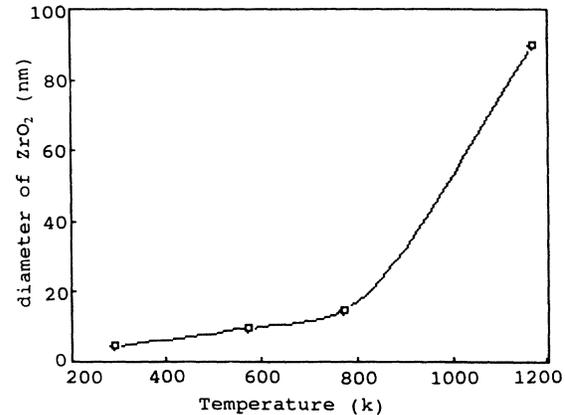
FIG. 2. The variation of the grain size with the annealing temperature.
