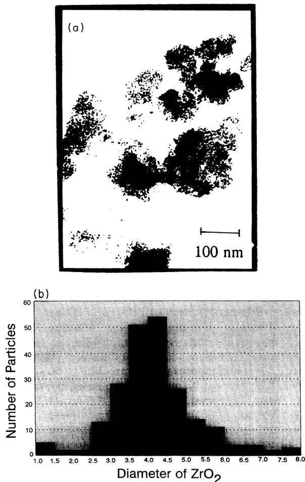
FIG. 1. (a) TEM micrograph of 5-nm diameter  $\text{ZrO}_2$  nanoclusters. (b) The distribution of the diameters of the  $\text{ZrO}_2$  nanoclusters.
