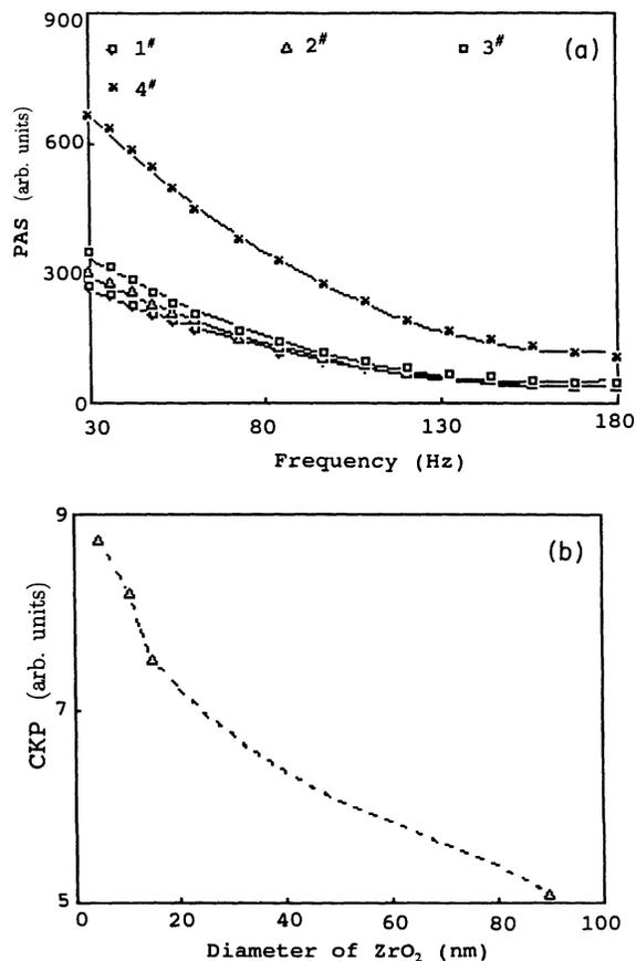
FIG. 4. (a) The variation of the PAS signal with the frequency. (b) The variation of the thermal constants with the diameter of the  $\text{ZrO}_2$  nanoclusters.
