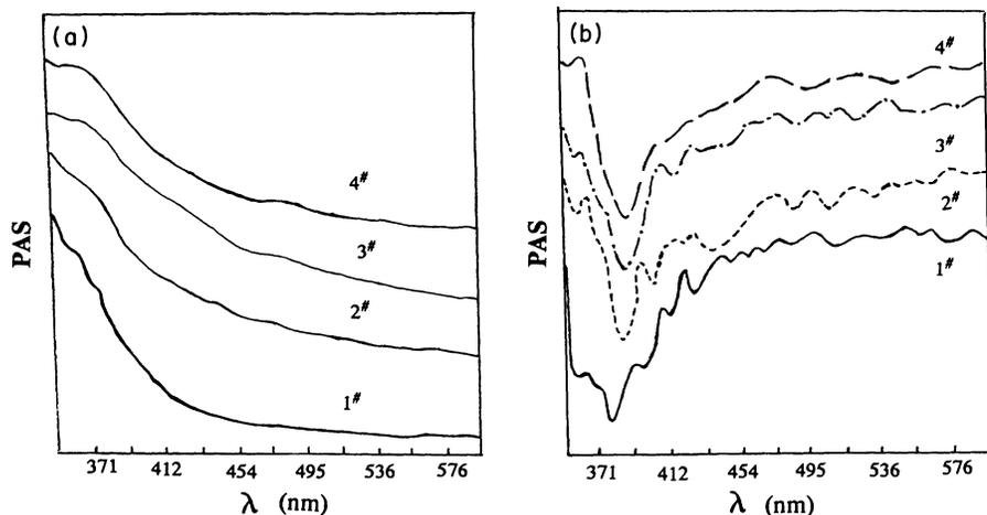
FIG. 3. The PAS (a) and the first-order differential PAS (b) of the  $\text{ZrO}_2$  nanoclusters of different average size. #1: 5 nm; #2: 10 nm; #3: 15 nm; #4: 90 nm.
