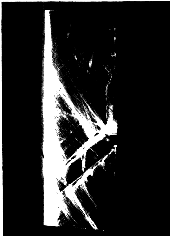
FIG. 1. (a) Schematic drawing of an X cut of the crystal, showing the regions which were sawed for the samples S1 and S2 . (b) X-ray topograph of an X cut of the crystal with high density (15 000 ppm) of impurities.
