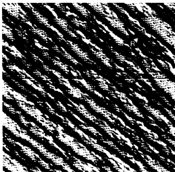
FIG. 1. A 600 \text{ Å} \times 600 \text{ Å} STM topograph of a vicinal Si(111) cut 4^\circ off the [111] towards [11 \bar{2} ]. The surface was produced by flashing the sample twice to 1280°C for 20 s, followed by quench cooling (Ref. 35). The arrow, labeled R, indicates rising step edges in the [\bar{1}\bar{1}2] direction. The tunneling current was 1 nA for a sample bias of +2 V. The image is nine point smoothed and differentiated to highlight the step edges.
