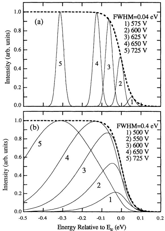
FIG. 4. Simulation of the dependence of band TED's on applied voltage for (a) a narrow and (b) a wide Gaussian band. This demonstrates how narrow bands pass through  $E_F$  while for a wide band, the emission remains near  $E_F$ . ( $E_{B0} = 1.5$  eV,  $\gamma = 0.0025$  eV/V,  $T = 300$  K).
