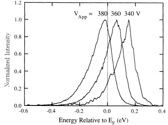
FIG. 6. FEES spectra as a function of applied field from a high clean nanometric protrusion formed on a W field emitter. For the lower voltages the peak shifts to above  $E_F$ .
