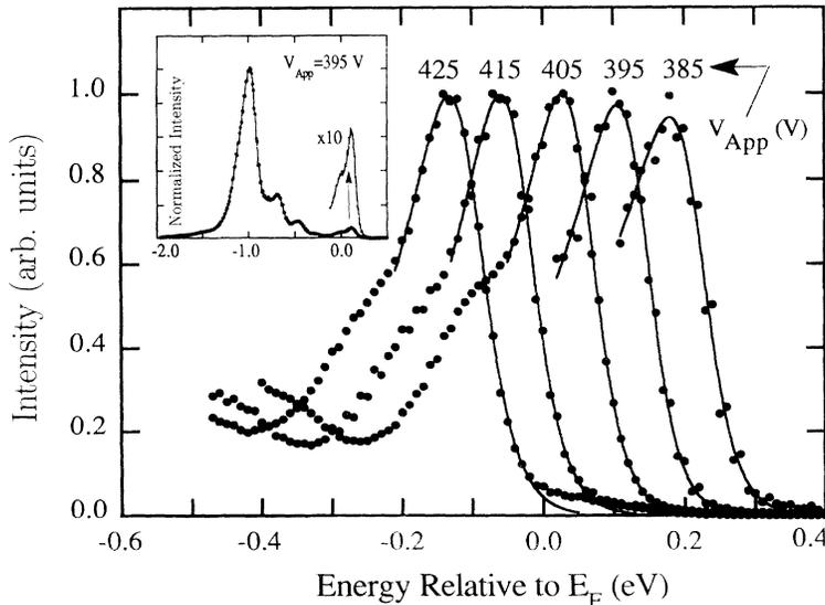
FIG. 2. The high-energy peak versus  $V_{App}$  of TED's from a high nanometric protrusion formed on a W field emitter with adsorption at the protrusion apex. Inset: full spectra for one fixed voltage. The high-energy peak passes through  $E_F$  upon variation of the applied field.
