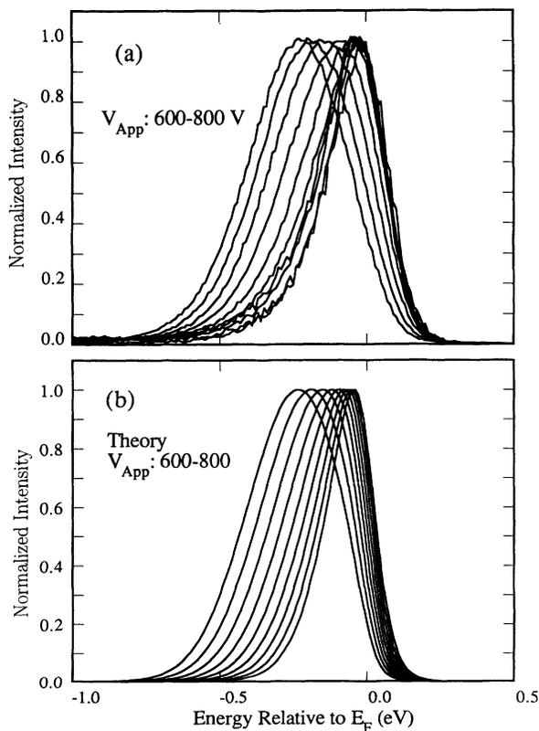
FIG. 3. (a) FEES spectra as a function of applied field from a relatively small nanometric protrusion formed on a W field emitter. (b) Calculation of TED's using equation in the text and parameters determined from Fig. 3(a).
