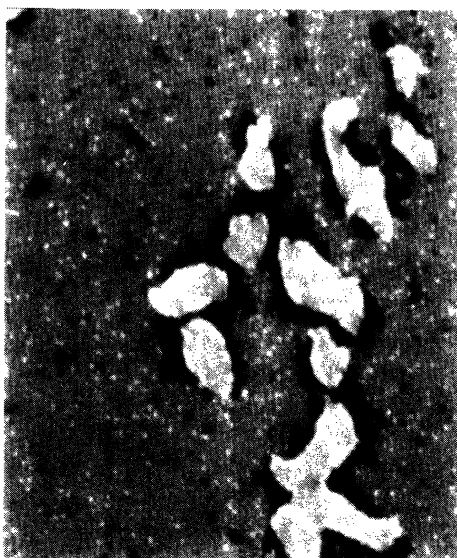
FIG. 9. Hole-island pairs interacting on a terrace. Note a number of small dark holes and bright dots on the terrace. Also apparent is the presence of ridges around the edges of the islands ( 1547 \times 1234 \text{ \AA}^2 , I = 0.8 \text{ nA} , V = -0.9 \text{ V} ).
